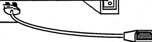
The GO Quick Charger connects to the GO computer to quickly recharge its battery and to provide AC power for computer operation. The Quick Charger snaps together with the GO Floppy Disk Drive to provide power for simultaneous computer and disk drive operation. The Quick Charger also provides ports that can connect the GO computer with serial printers and RS232 devices, AppleTalk and TOPS networks, PC or Macintosh computers, and an AT computer keyboard.
