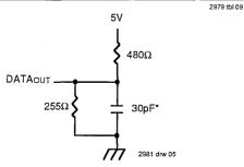
Figure 1. AC Test Load
