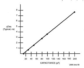
Figure 3. Lumped Capacitive Load, typical Derating
