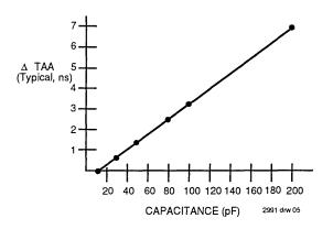
Figure 3. Lumped Capacitive Load, typical Derating
