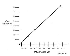
Figure 3. Lumped Capacitive Load, typical Derating
