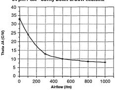
Measurements were done using Temp09 Delco Thermal Die (.250sq.)
