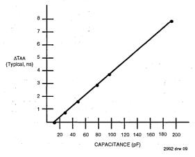
Figure 3. Lumped Capacitive Load, typical Derating
