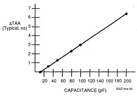
Figure 3. Lumped Capacitive Load, Typical Derating
