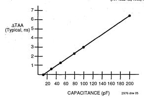
Figure 3. Lumped Capacitive Load, Typical Derating
