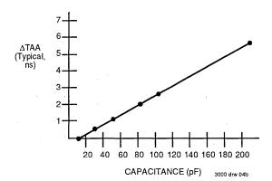
Figure 3. Lumped Capacitive Load, Typical Derating
