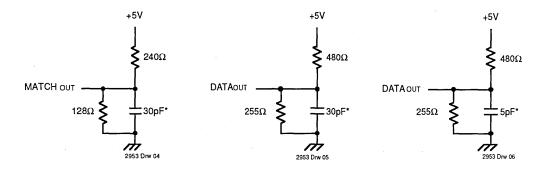
Figure 1. AC Test Load for MATCH
