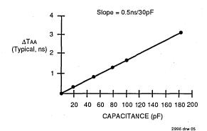
Figure 3. Lumped Capacitive Load, Typical Derating Curve
