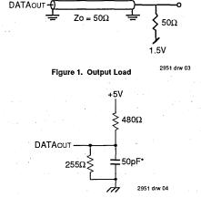
Figure 2. Output Load (for tohz, tchz, tolz and tclz) \*including scope and jig
