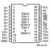
DIP/SOIC/CERPACK/SOJ TOP VIEW
