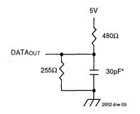
Figure 1. AC Test Load
