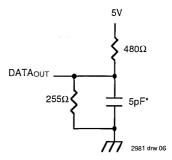
Figure 2. AC Test Load (for tclz, tchz, twhz and tow)
