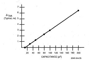
Figure 3. Lumped Capacitive Load, typical Derating
