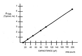
Figure 3. Lumped Capacitive Load, typical Derating
