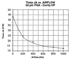
Measurements were done using Temp09 Delco Thermal Die (.250sq.)
