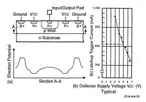
Figure 5. IDT CMOS Latchup Suppression
