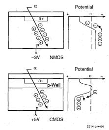
Figure 4. IDT CMOS Built-In High Alpha Particle Immunity
