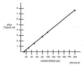
Figure 3. Lumped Capacitive Load, typical Derating
