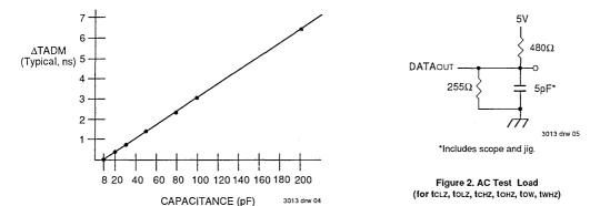
Figure 1A. Lumped Capacitive Load **Typical Derating Curve**
