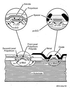
Figure 3. IDT CMOS Device Cross Section
