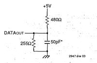
Figure 1. Output Load
