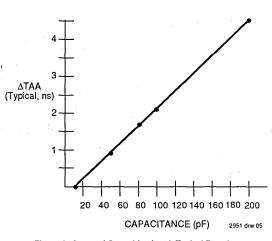
Figure 3. Lumped Capacitive Load, Typical Derating
