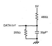
Figure 1. AC Test Load
