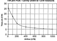
Measurements done with Delco Temp09 Thermal Die (.250"sq.)
