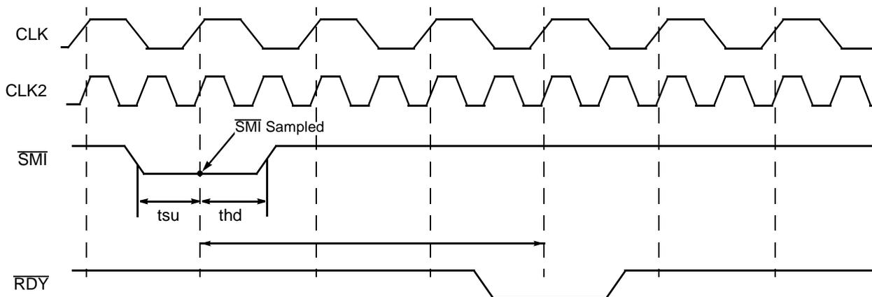
Figure 24. SMI Timing for Servicing an I/O Trap
