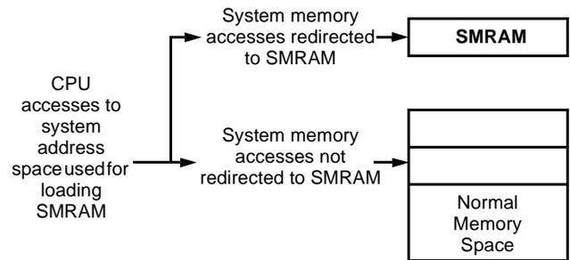
Figure 26. Redirecting System Memory Address to SMRAM
