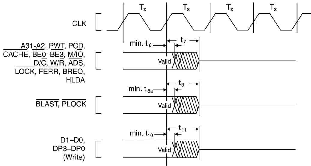
Figure 41. Maximum Float Delay Timing
