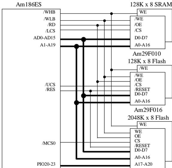
Figure 2. The Am186ES with extended single banked Flash and SRAM memory
