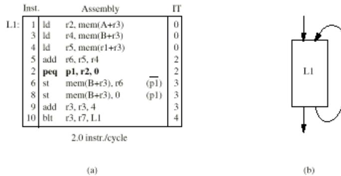
Figure 4. Forming larger blocks using predication, (a) assembly code, (b) control flow graph.
