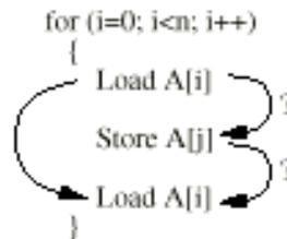
Figure 12. Redundant load elimination example.
