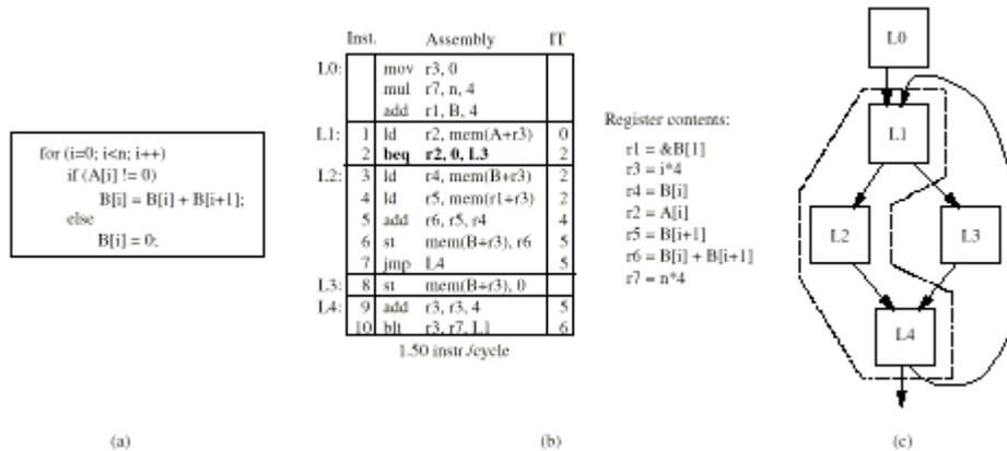
Figure 1. Traditional Compilation example (a) original Loop, (b) assembly code, (c) control flow graph.
