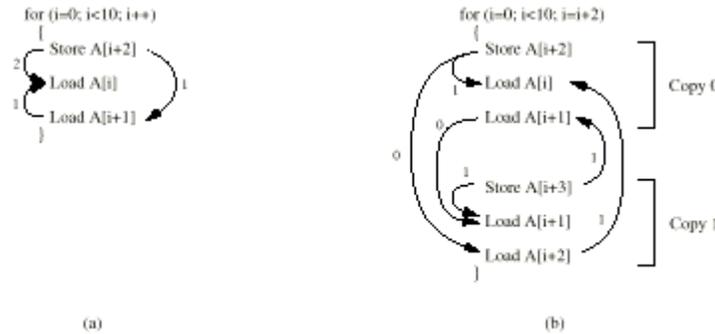
Figure 13. Loop unrolling example, (a) original code, (b) code after loop unrolling.
