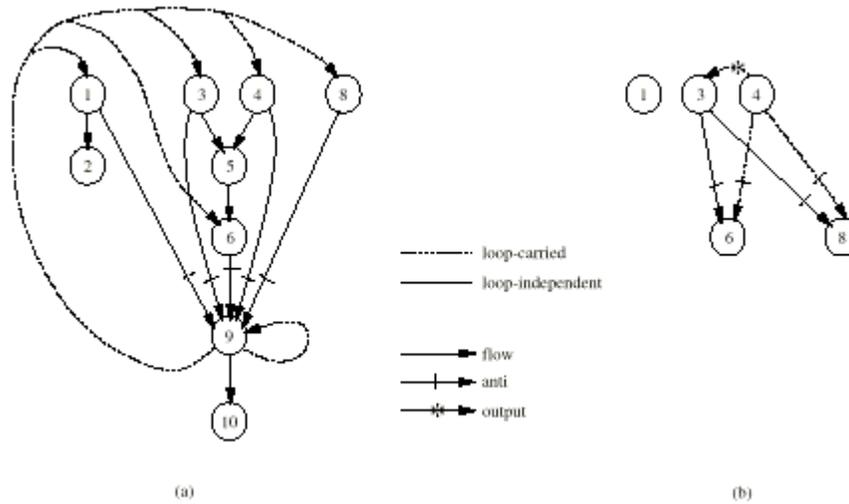
Figure 2. Dependence graphs for example loop; (a) register dependences, (b) memory dependences.
