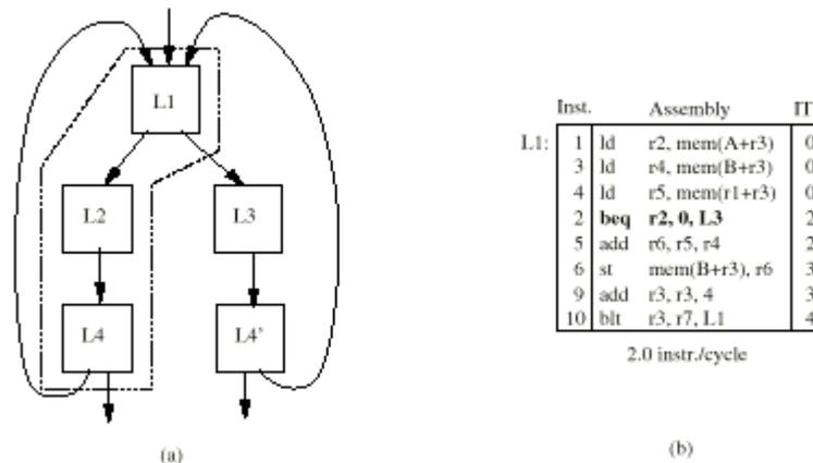
Figure 3. Forming larger blocks from traces, (a) control flow graph, (b) assembly code for the *then* path.
