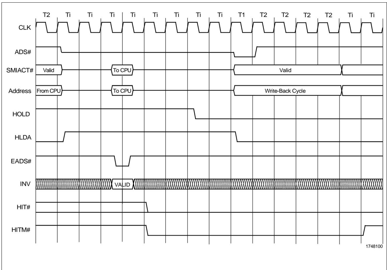
Figure 3-27. Hold Inquiry that Hits on a Modified Data Line
