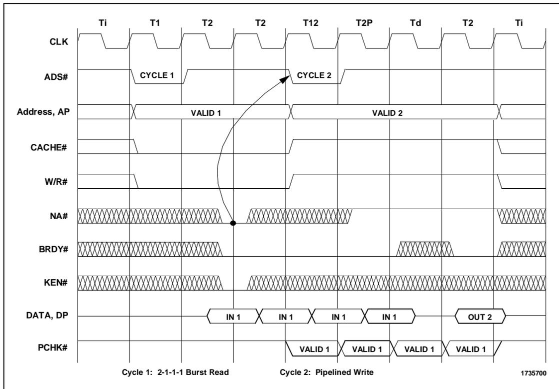
Figure 3-12. Read Cycle Followed by Pipelined Write Cycle
