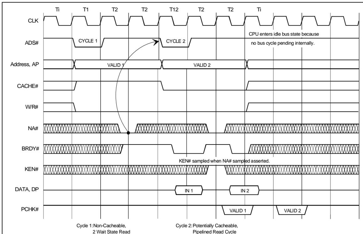
Figure 3-10. Pipelined Single Transfer Read Cycles
