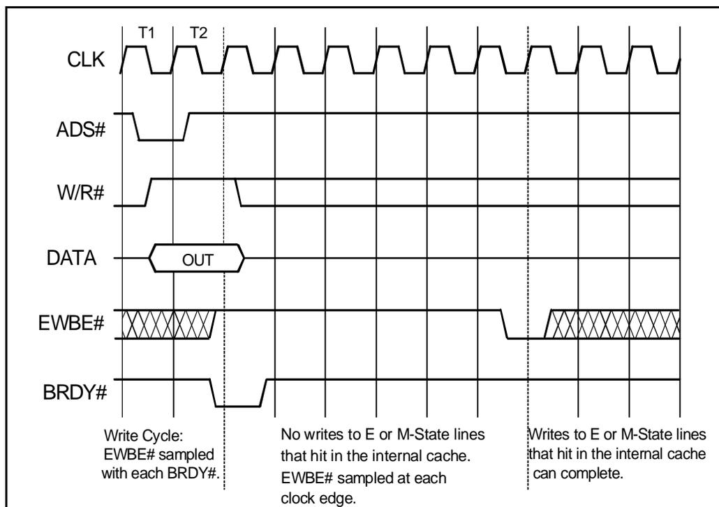
Figure 3-17. External Write Buffer Empty (EWBE#) Timing
