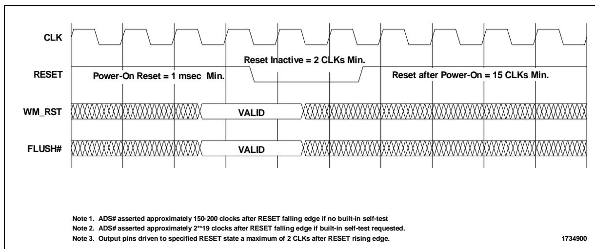
Figure 3-2. RESET Timing
