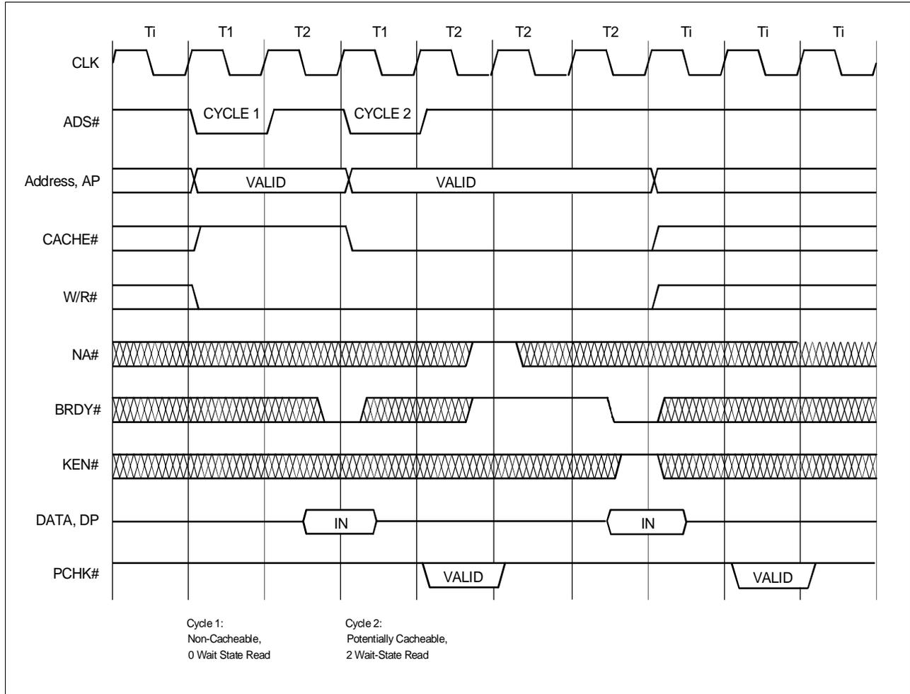
Figure 3-4. Non-Pipelined Single Transfer Read Cycles
