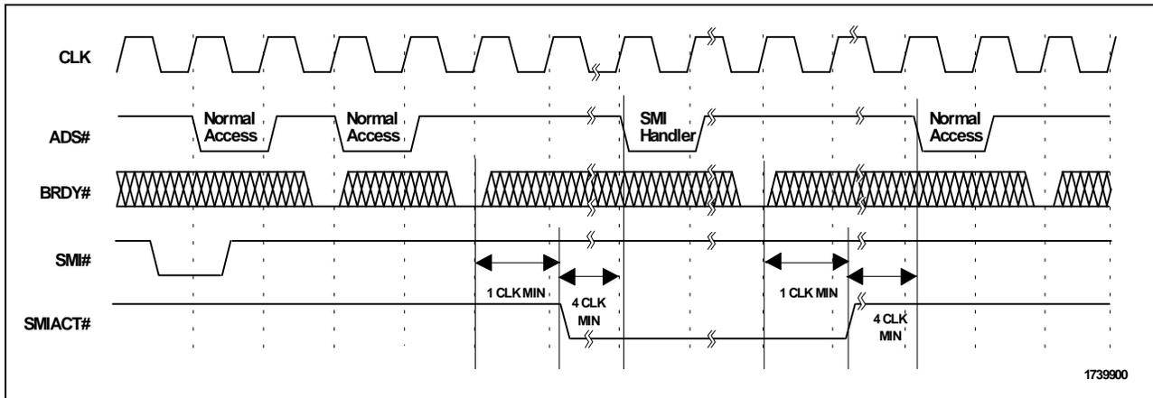
Figure 3-14. SMIACT# Timing in SL Compatible Mode
