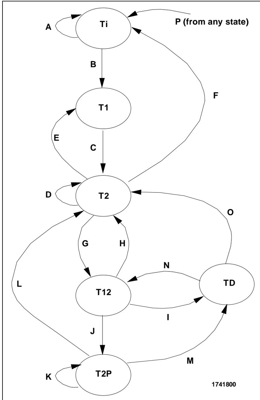
Figure 3-3. IBM 6x86MX CPU Bus State Diagram
