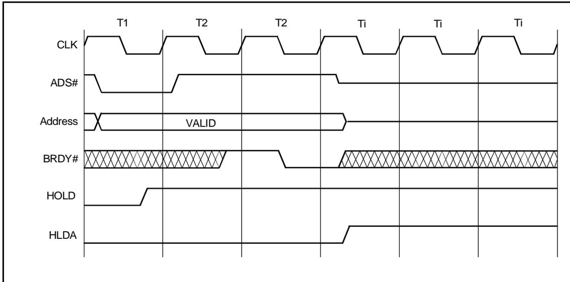
Figure 3-19. Requesting Hold During a Non-Pipelined Bus Cycle
