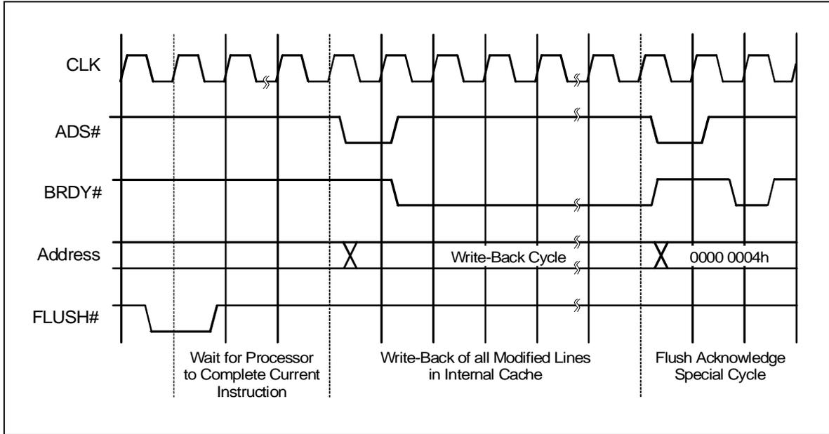
Figure 3-16. Cache Invalidation Using FLUSH#
