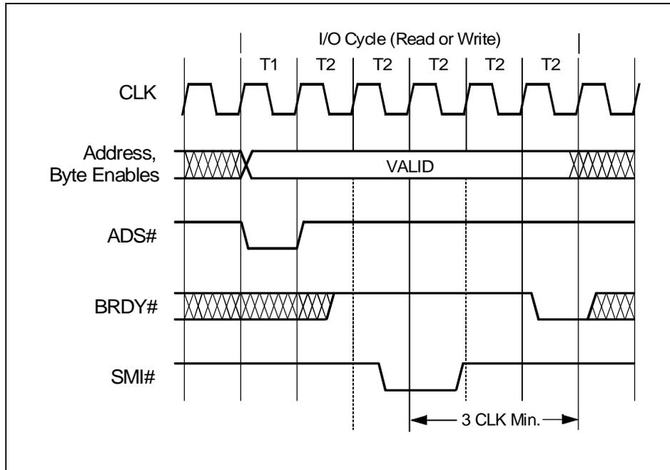
Figure 3-15. SMM I/O Trap Timing
