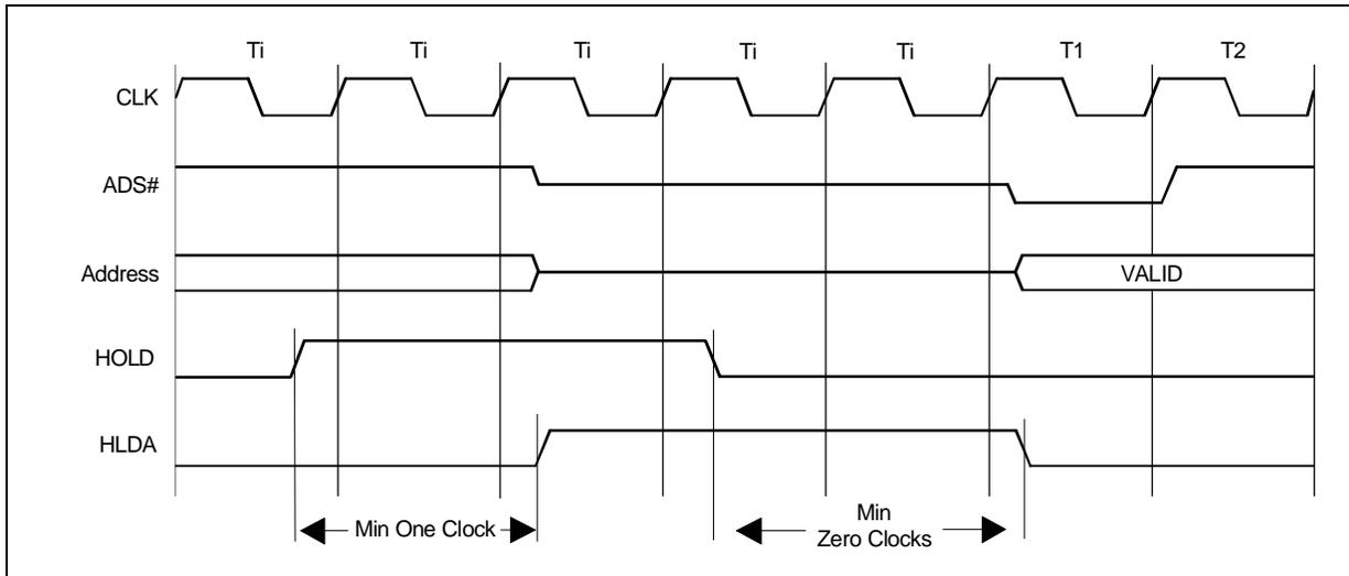
Figure 3-18. Requesting Hold from an Idle Bus
