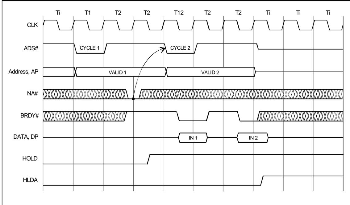
Figure 3-20. Requesting Hold During a Pipelined Bus Cycle
