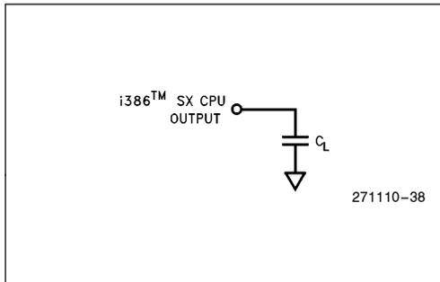
Figure 7.2. AC Test Loads
