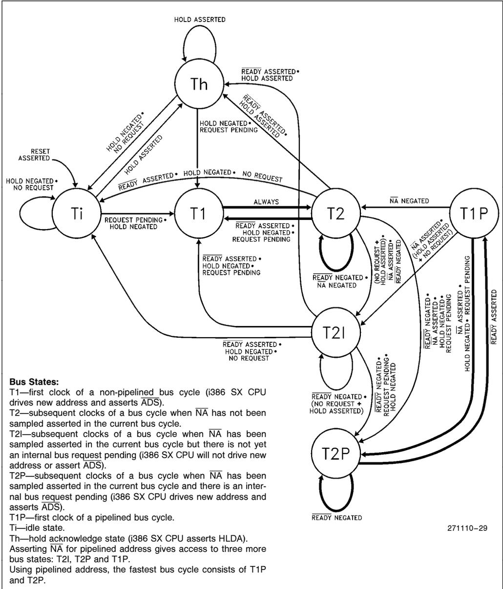
Figure 5.12. Complete Bus States (including pipelined address)
