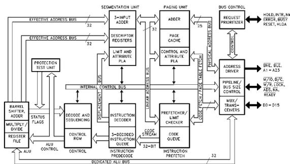
**i386™ SX Pipelined 32-Bit Microarchitecture**
