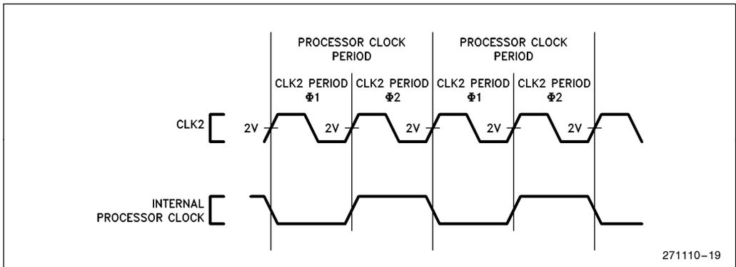
**Figure 5.2. CLK2 Signal and Internal Processor Clock**
