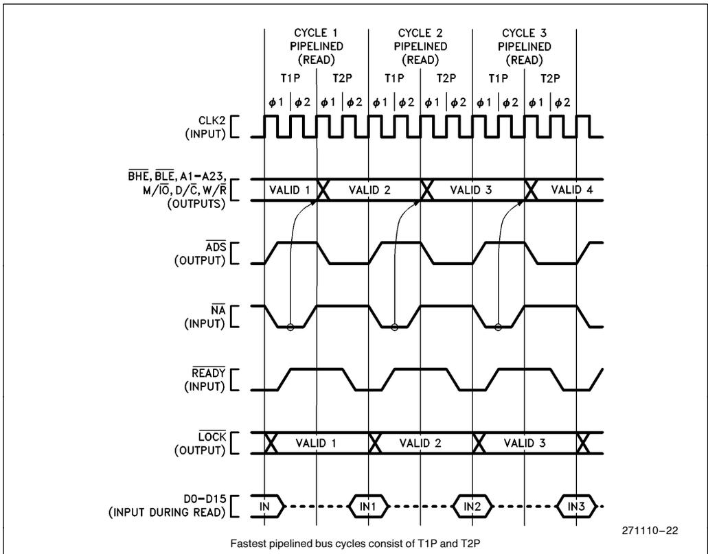
**Figure 5.5. Fastest Read Cycles with Pipelined Address Timing**
