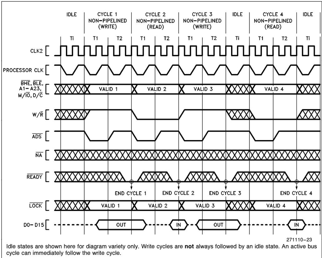
Idle states are shown here for diagram variety only. Write cycles are **not** always followed by an idle state. An active bus cycle can immediately follow the write cycle.
