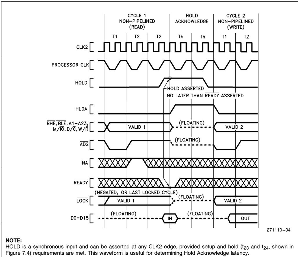
**Figure 5.17. Requesting Hold from Active Bus ( $\overline{NA}$  inactive)**
