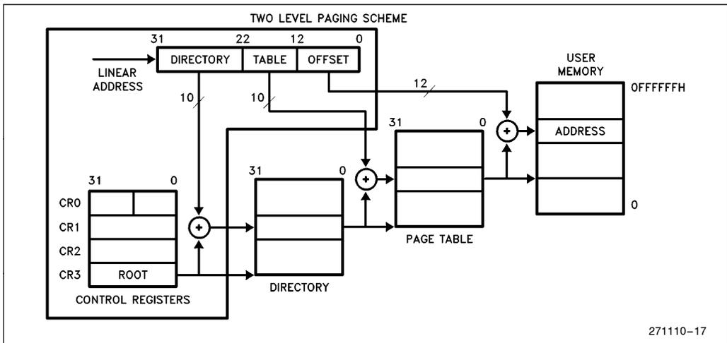
**Figure 4.10. Paging Mechanism**
