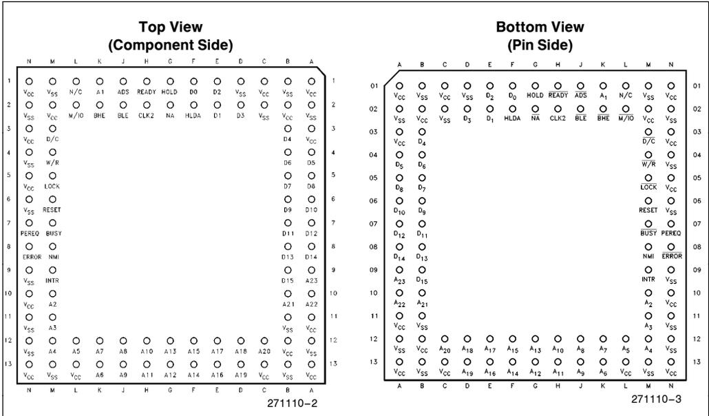
**Figure 1.1. i386™ SX 88-Lead Pin Grid Array Pinout**
