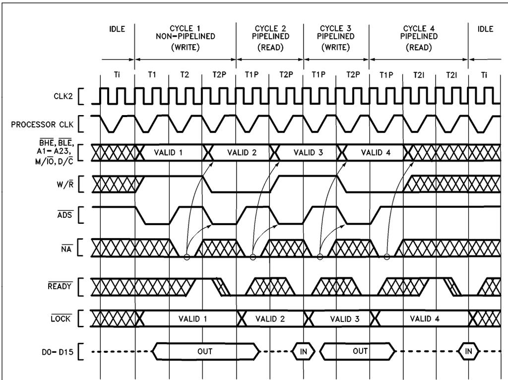
Following any bus state (Ti) the address is always non-pipelined and  $\overline{NA}$  is only sampled during wait states. To start address pipelining after an idle state requires a non-pipelined cycle with at least one wait state (cycle 1 above). The pipelined cycles (2, 3, 4 above) are shown with various numbers of wait states.
