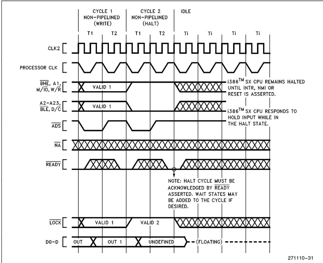
**Figure 5.14. Example Halt Indication Cycle from Non-Pipelined Cycle**
