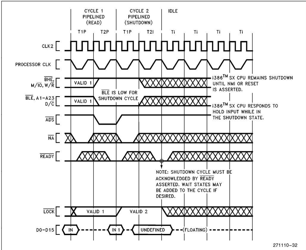
Figure 5.15. Example Shutdown Indication Cycle from Pipelined Cycle
