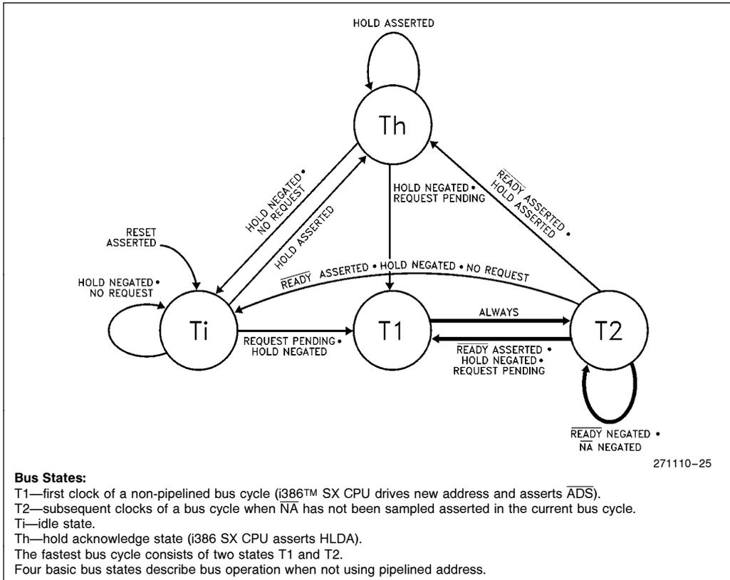
**Figure 5.8. Bus States (not using pipelined address)**
