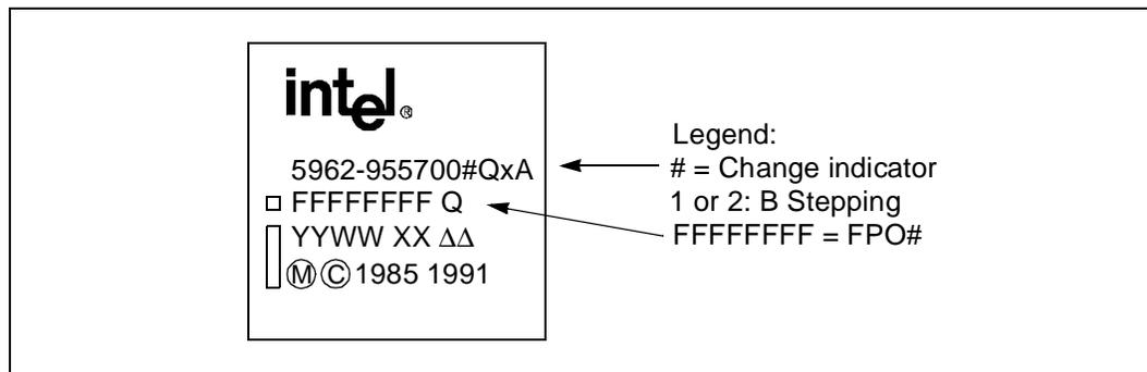
If there is not an FPO# line on the device — hence, no change indicator — but is marked with a Qxxxx (where x=any digit) on the second line, it is likely a pre-production sample part. Consult your Intel representative if you are unclear on the device stepping.
