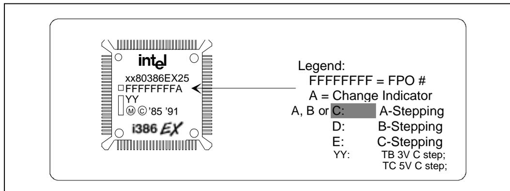
The B-stepping production version of the Special Environment Intel386 EX is designated with a change indicator of '1' or '2'. Figure 2 is an illustration indicating where the change indicator marking is located on the package markings. The change indicator is used to relate information found here, and in other documents like datasheets, to a specific device.
