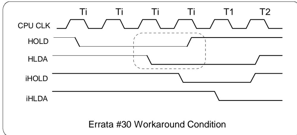
Another workaround is to delay the generation of HOLD until the last T2-state of a valid bus cycle (excluding refresh cycles or INTA cycles).
