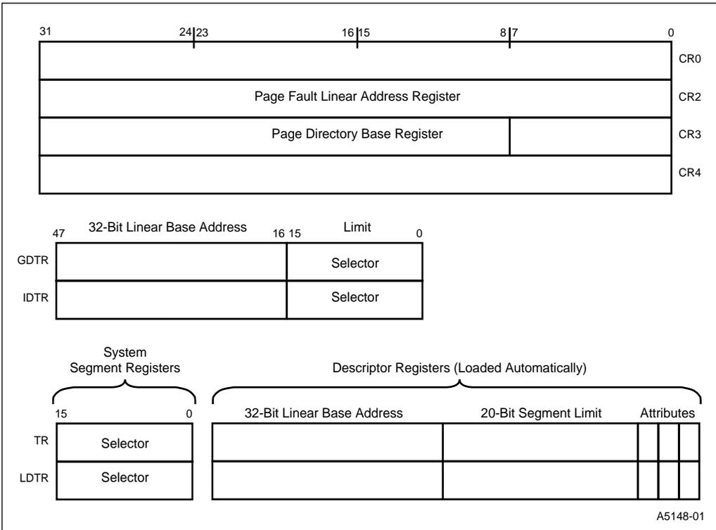
Figure 4-4. System-Level Registers
