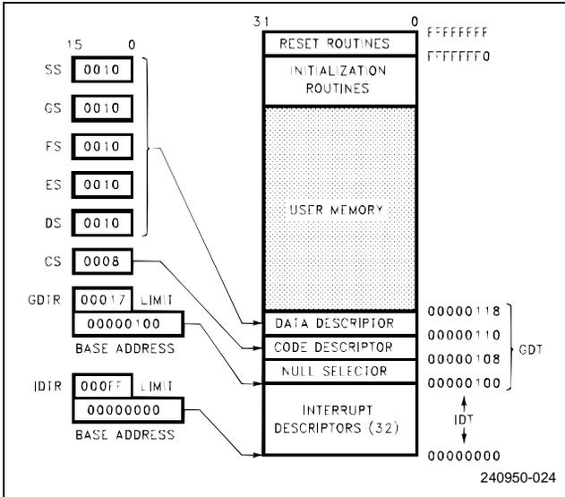
Figure 6-17. Simple Protected System
