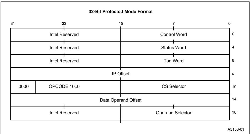
**Figure 4-10. Protected Mode FPU Instructions and Data Pointer Image in Memory—32-Bit Format**
