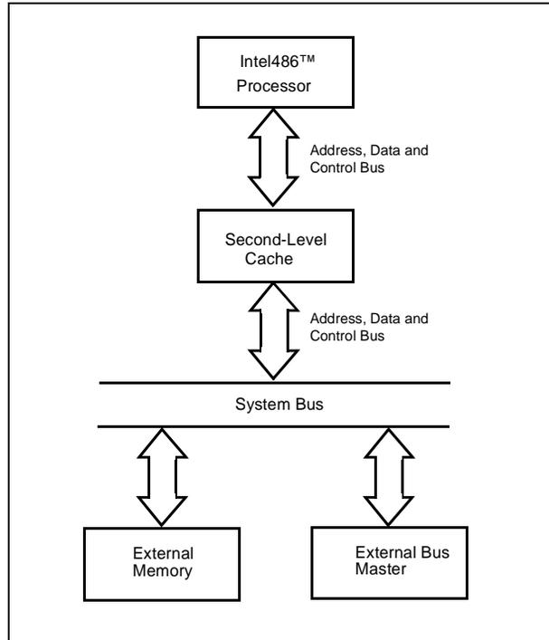
**Figure 10-27. System with Second-Level Cache**
