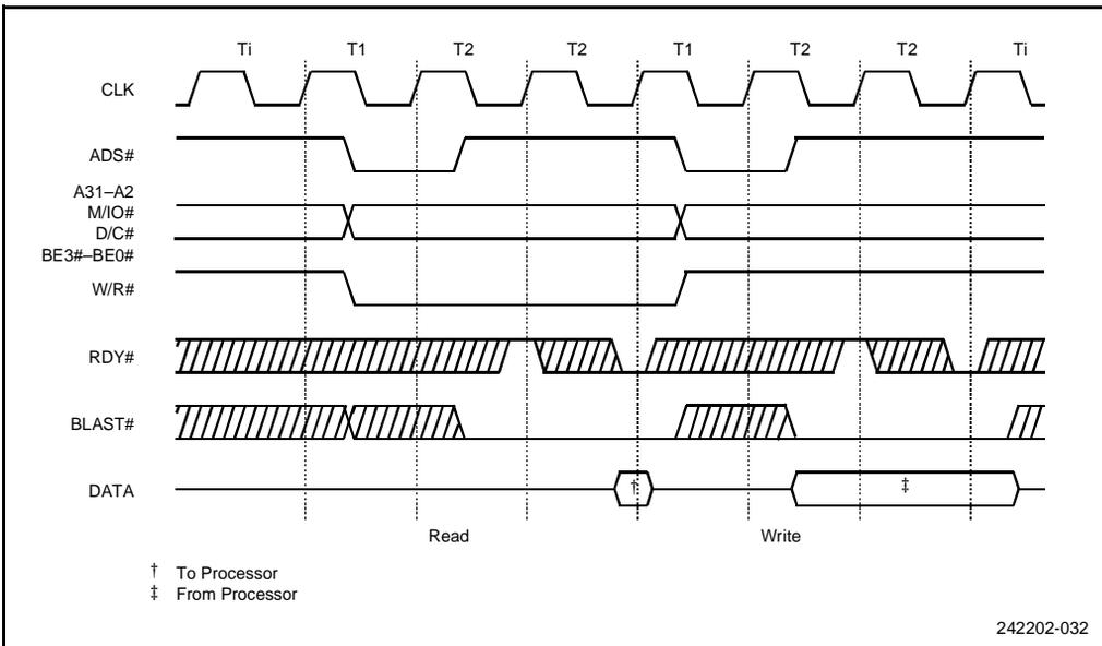
**Figure 10-11. Basic 3-3 Bus Cycle**
