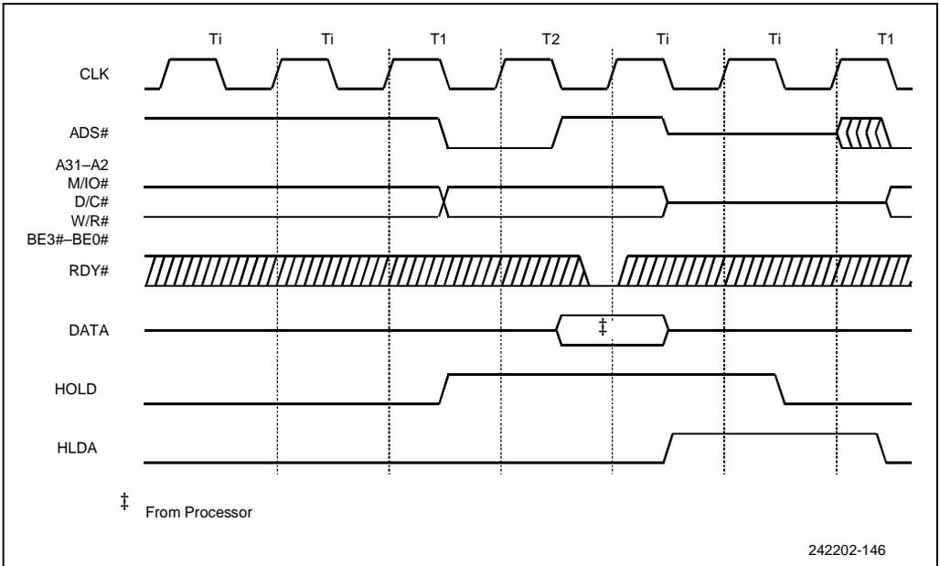
Figure 10-29. HOLD/HLDA Cycles
