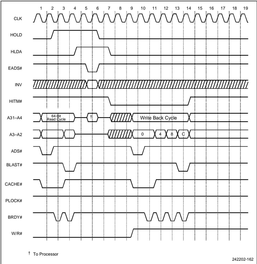
**Figure 10-50. Snoop under HOLD Overlaying Pseudo-Locked Cycle**
