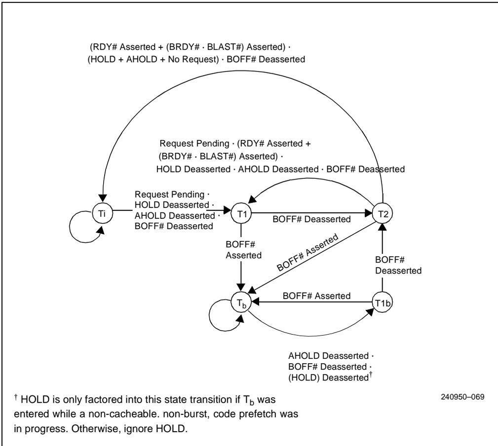
Figure 10-35. Bus State Diagram
