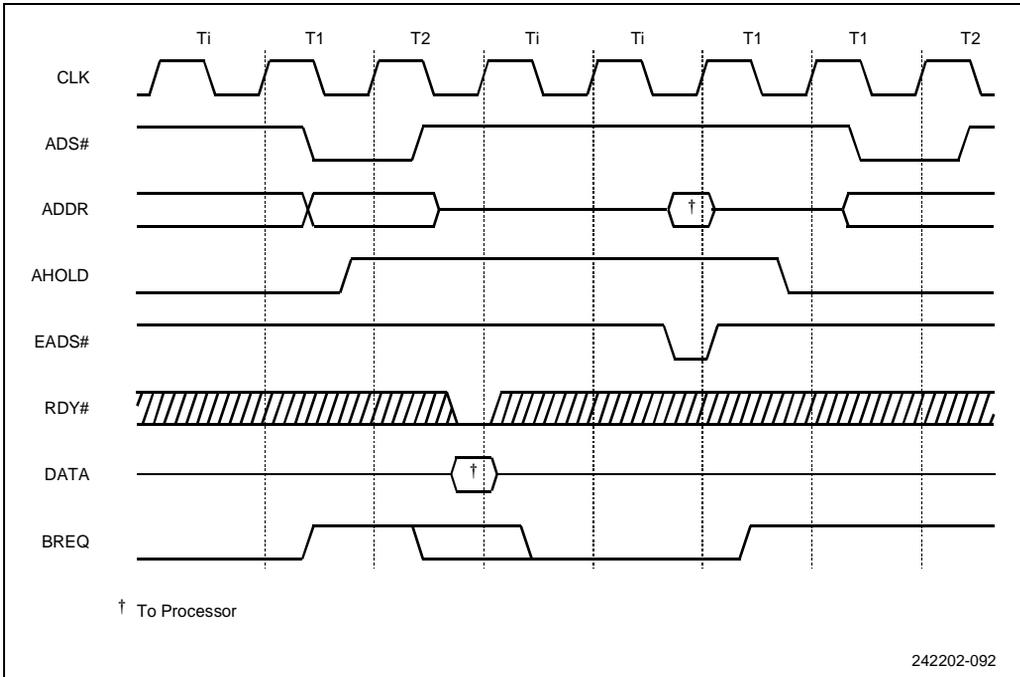
**Figure 10-26. Typical Internal Cache Invalidation Cycle**
