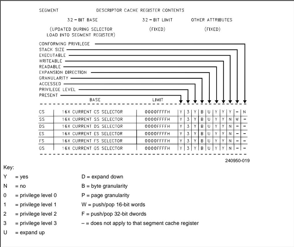
**Figure 6-12. Segment Descriptor Caches for Virtual 8086 Mode within Protected Mode (Segment Limit and Attributes are Fixed)**
