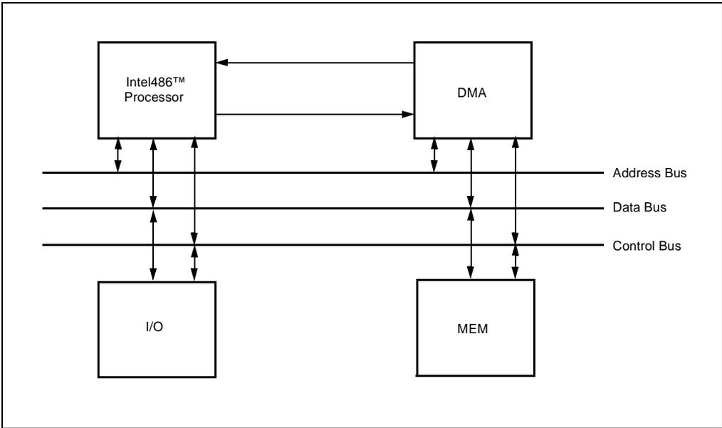
Figure 10-8. Single Intel486™ Processor with DMA
