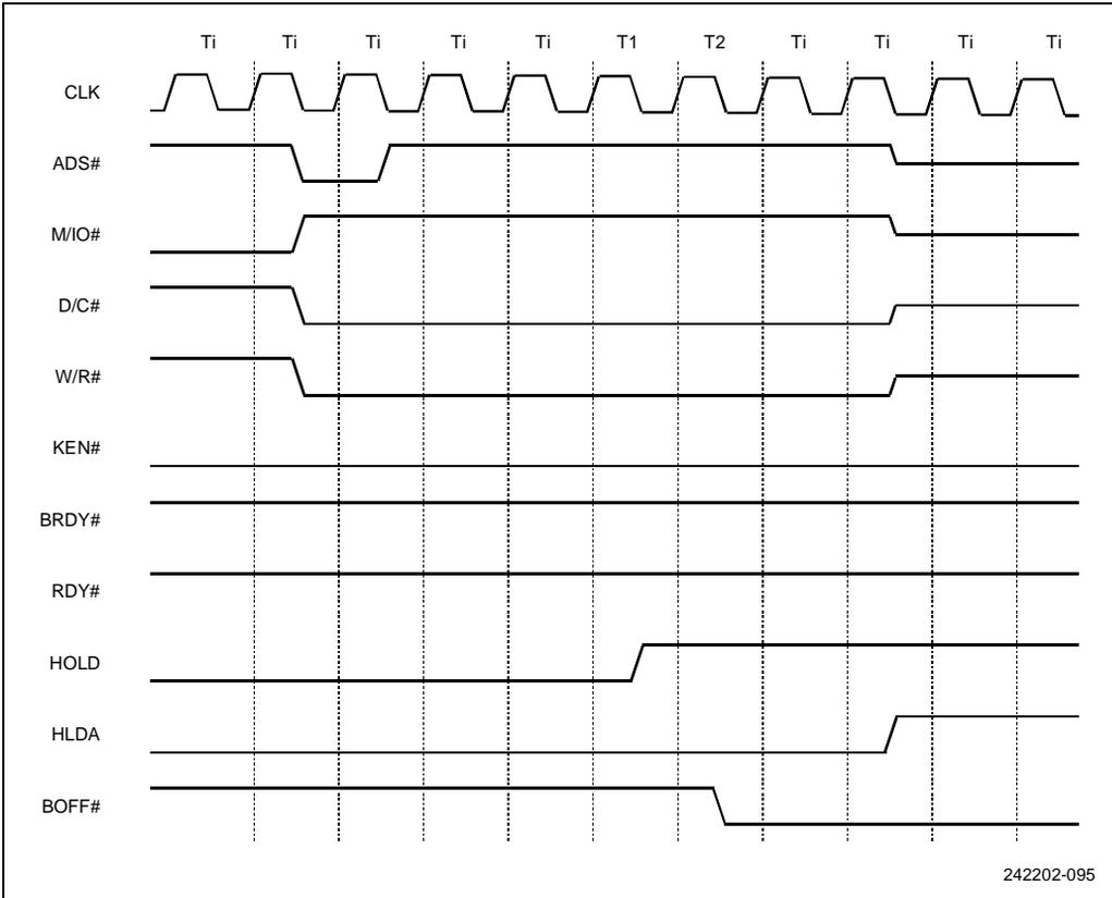
Figure 10-30. HOLD Request Acknowledged during BOFF#
