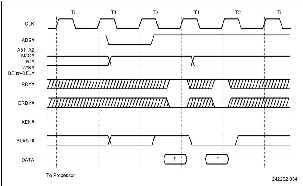
**Figure 10-13. Non-Cacheable Burst Cycle**
