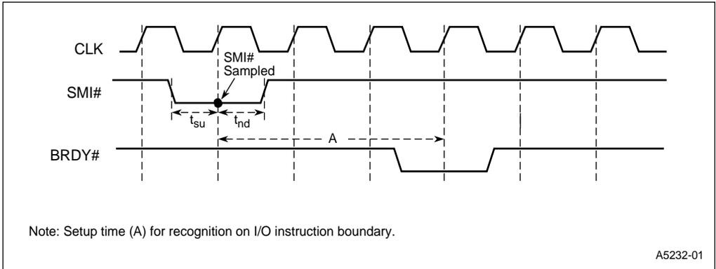
**Figure 8-3. SMI# Timing for Servicing an I/O Trap**
