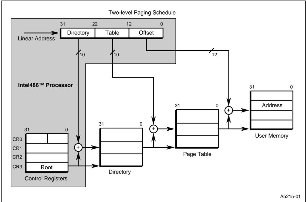
Figure 6-19. Paging Mechanism
