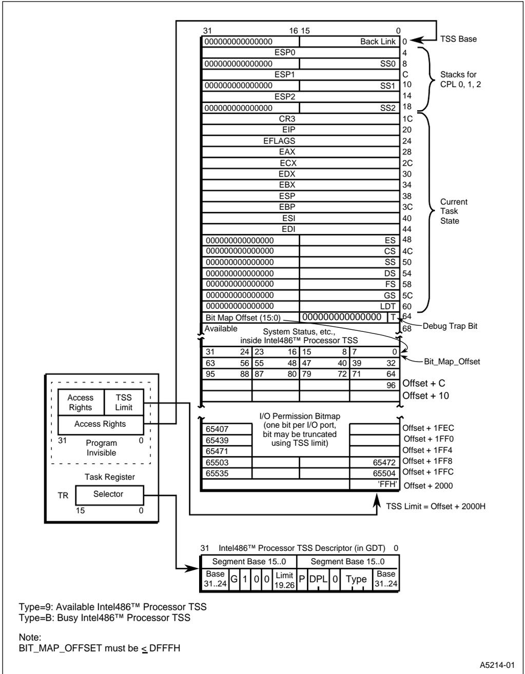
Figure 6-14. Intel486™ Processor TSS and TSS Registers
