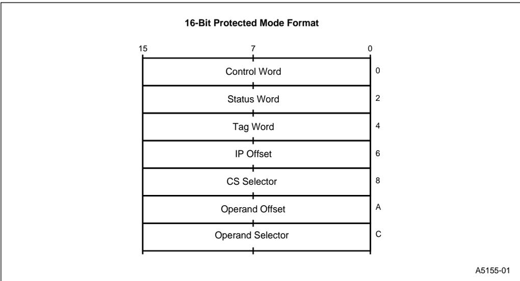
**Figure 4-12. Protected Mode FPU Instruction and Data Pointer Image in Memory—
