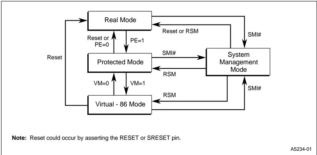
**Figure 8-6. Transition to and from System Management Mode**
