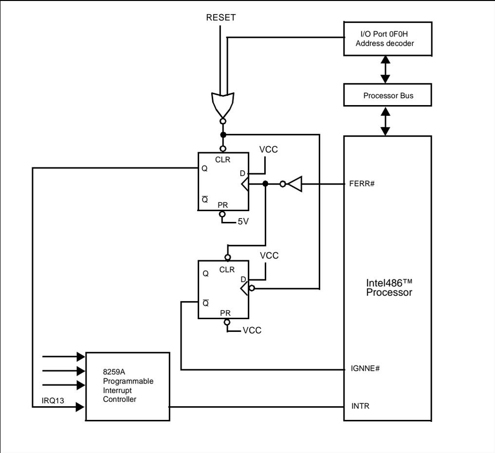
Figure 10-36. DOS-Compatible Numerics Error Circuit
