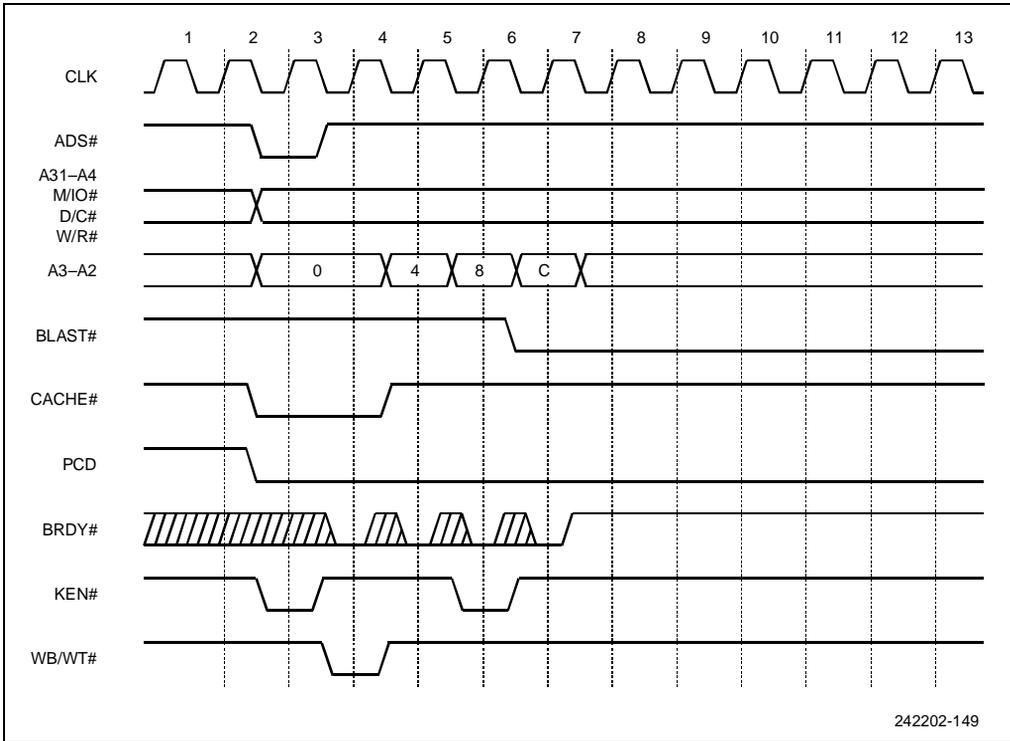
Figure 10-37. Basic Burst Read Cycle
