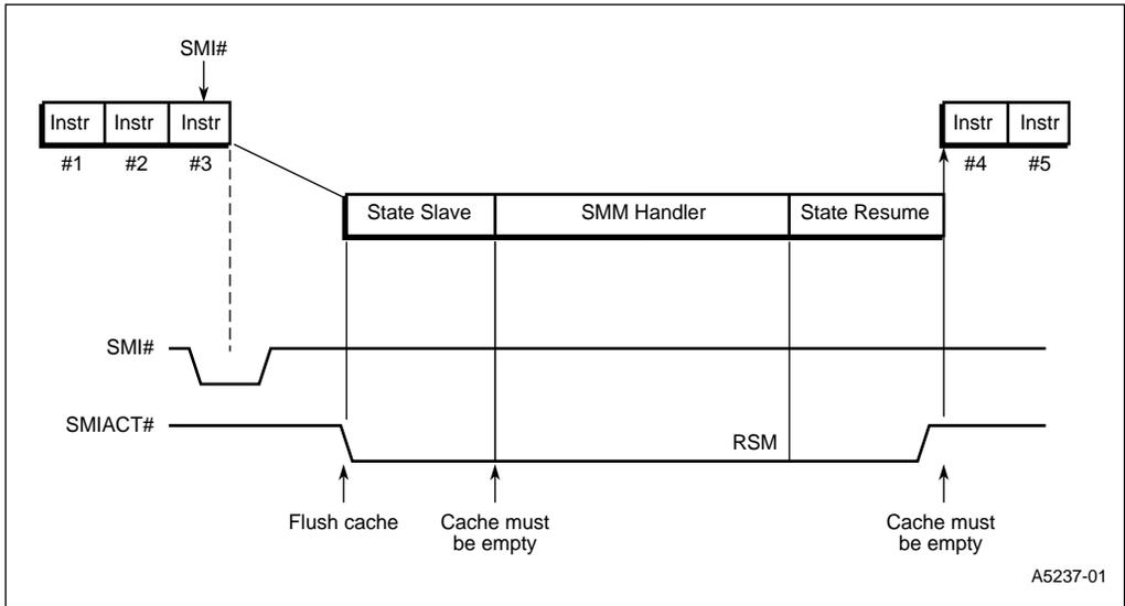
**Figure 8-13. FLUSH# Mechanism during SMM**
