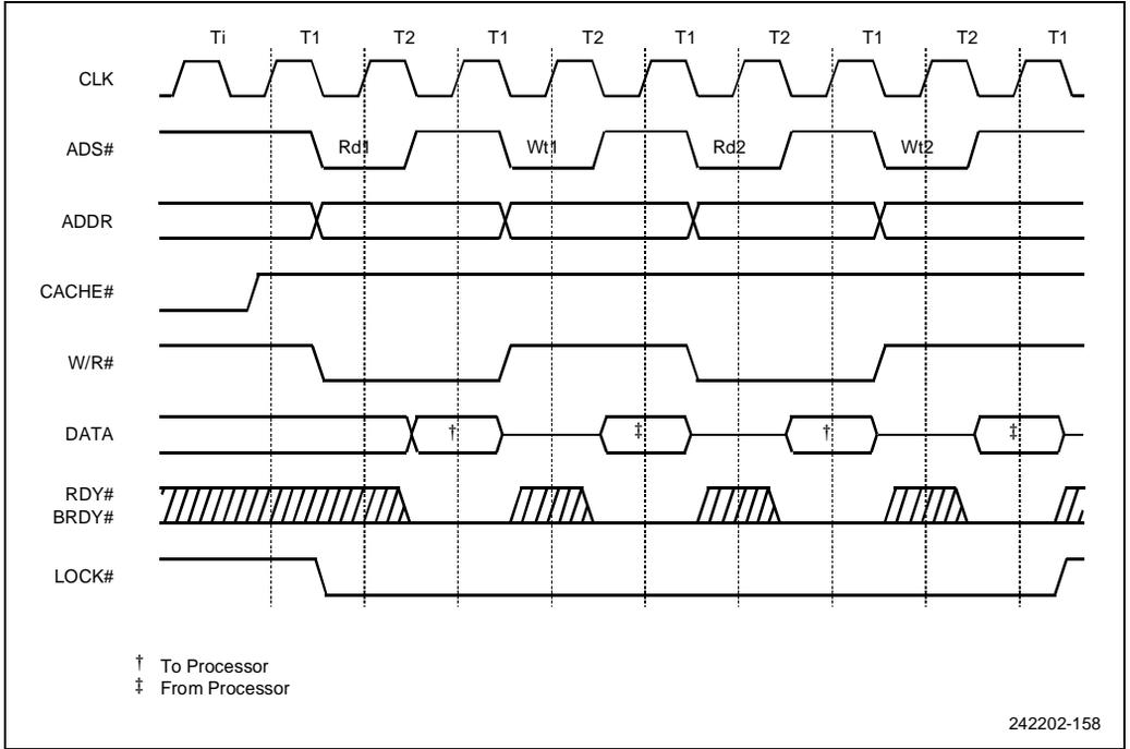
Figure 10-46. Locked Cycles (Back-to-Back)
