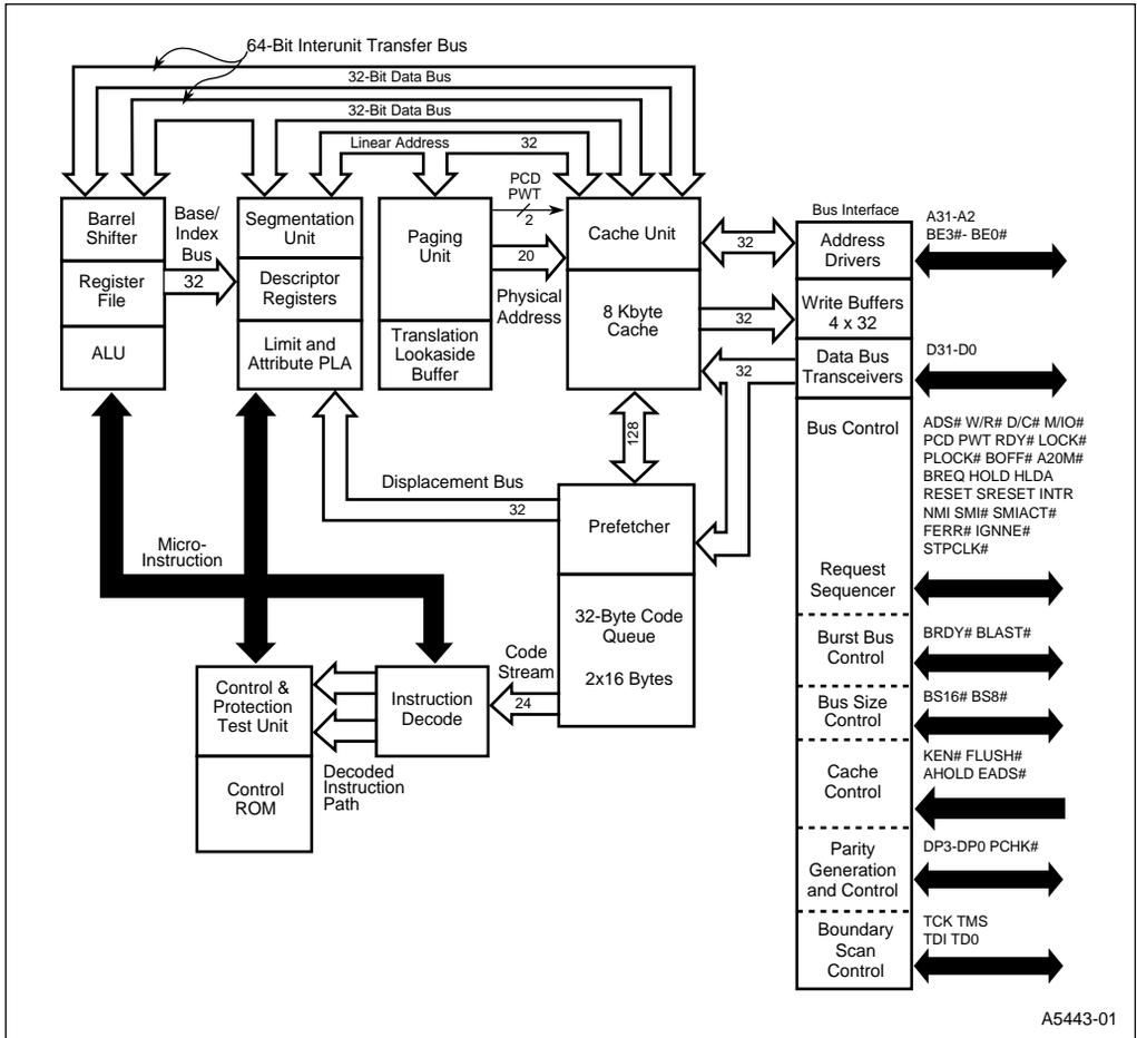
Figure 3-2. Intel486™ SX Processor Block Diagram
