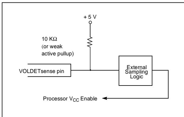
**Figure 9-4. Voltage Detect (VOLDET) Sense Pin**
