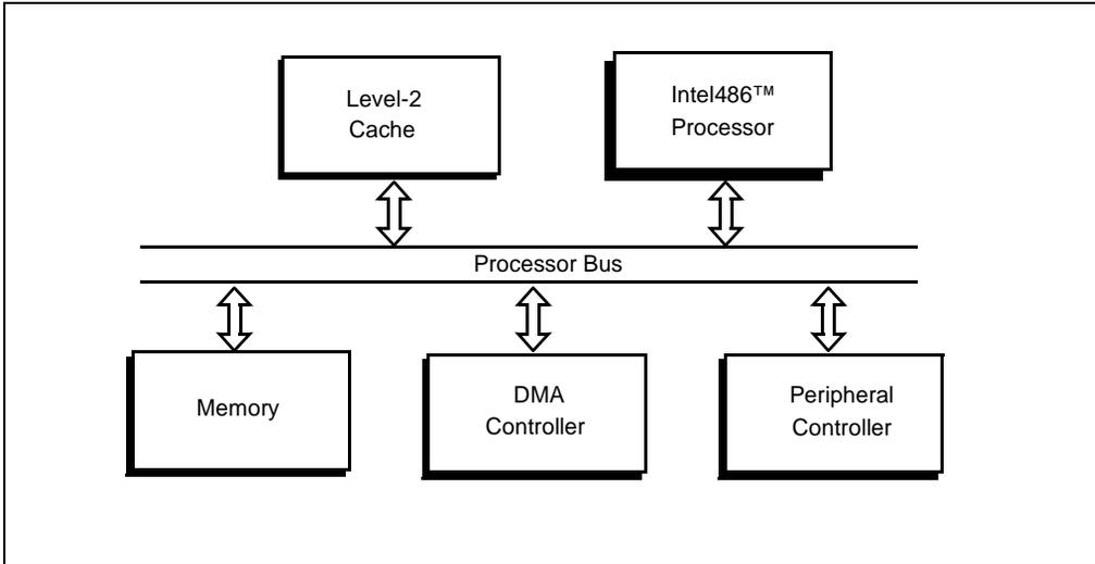
**Figure 3-10. Single-Processor System**
