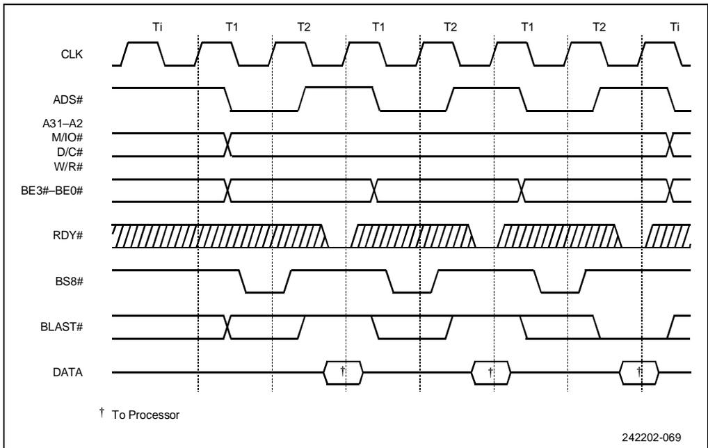
Figure 10-21. 8-Bit Bus Size Cycle
