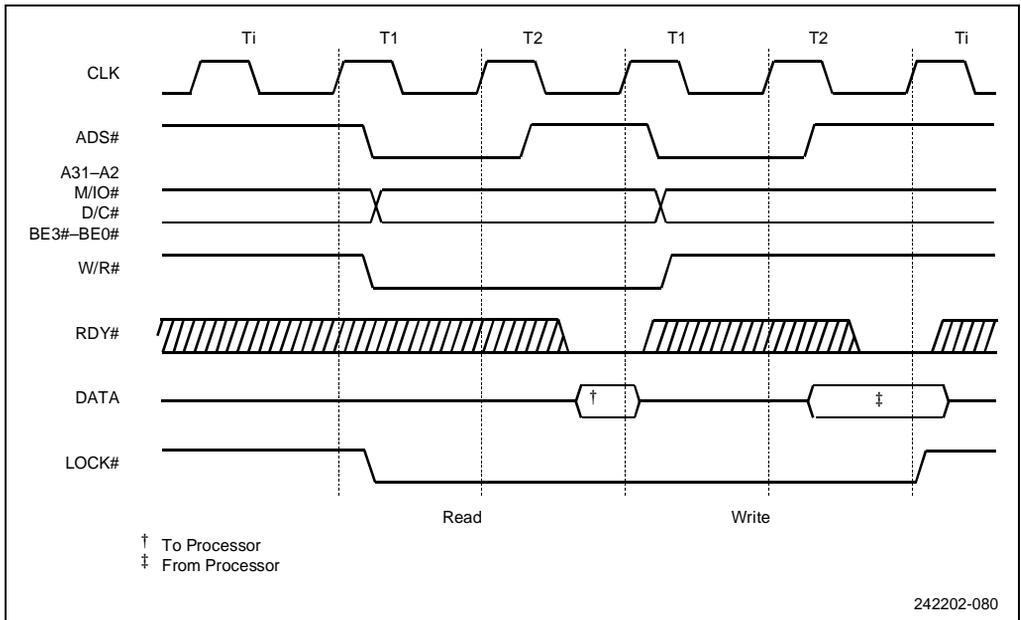
Figure 10-23. Locked Bus Cycle
