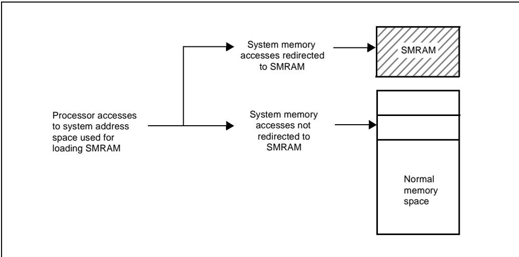
Figure 8-5. Redirecting System Memory Addresses to SMRAM
