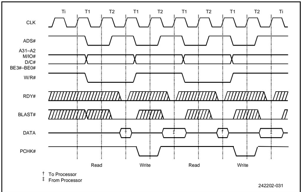
**Figure 10-10. Basic 2-2 Bus Cycle**
