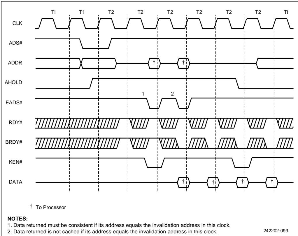
Figure 10-28. Cache Invalidation Cycle Concurrent with Line Fill
