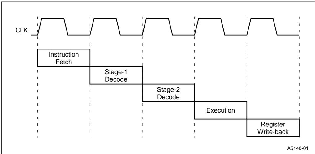
Figure 3-8. Internal Pipelining
