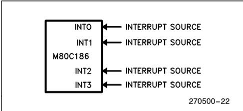
**Figure 22. Fully Nested (Direct) Mode Interrupt Controller Connections**
