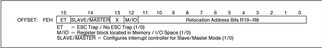
**Figure 9. Relocation Register**
