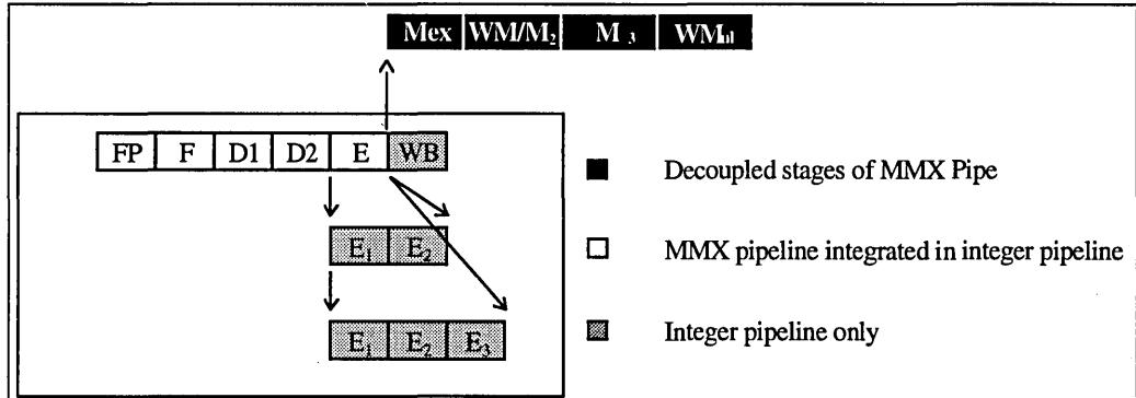
**Figure 2-1. MMX™ Pipeline Structure**
