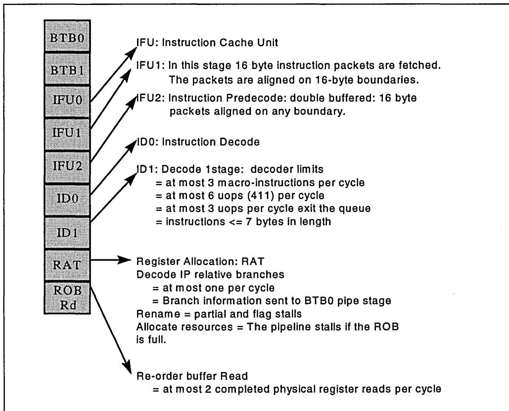
Figure 2-3. Out-Of-Order Core and Retirement Pipeline
