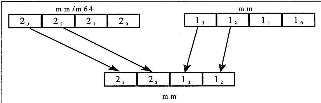
**Figure 5-4. Result of Non-Interleaved Unpack in MM1**
