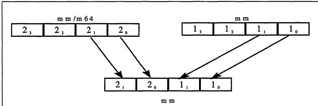
Figure 5-3. Result of Non-Interleaved Unpack in MM0
