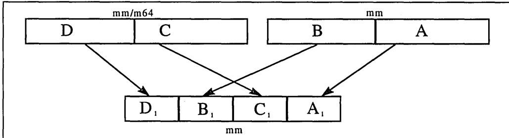
**Figure 5-2. Interleaved Pack with Saturation Example**
