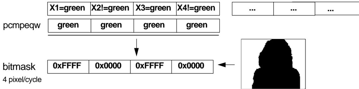
This mask is now used on the same four pixels from the picture with the woman and the equivalent four pixels from the Spring blossom. The “AND NOT” and “AND” instructions use the mask to identify which pixels to keep from the Spring blossom and the woman. They also turn the unwanted pixels to zeros. The “OR” instruction builds the final picture. Four pixels were mapped using only four MMX instructions without any branches.
