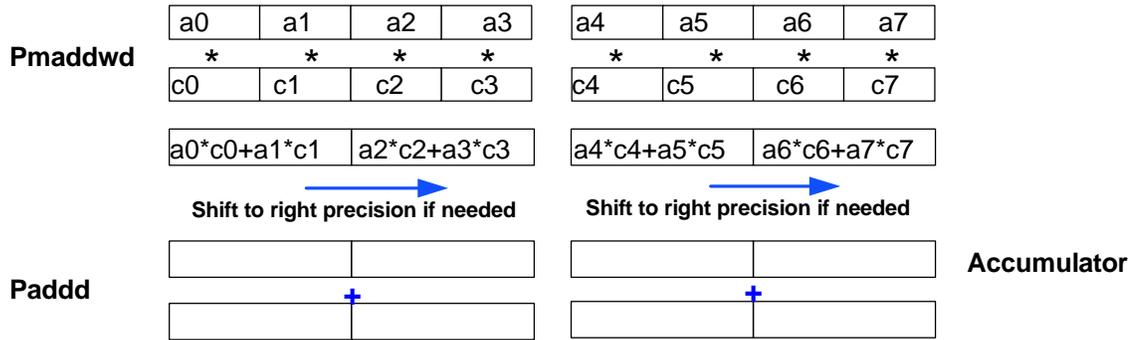
**Note:** Input data and coefficients are 16-bit precision. If not, first unpack to 16 bit.
