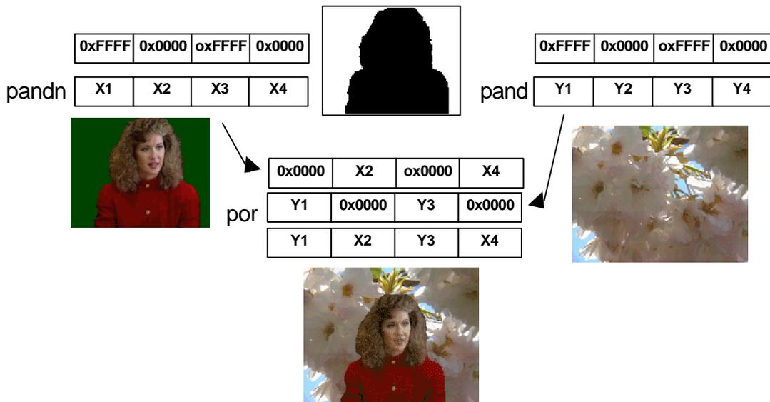
Without MMX technology, each pixel is processed separately and requires a conditional branch. Using MMX instructions, eight 8-bit pixels can be processed in parallel and no conditional branches are involved.
