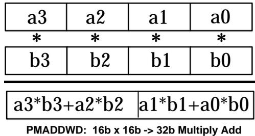
The PMADD instruction starts from a 16-bit, packed data type and generates a 32-bit packed, data type result. It multiplies all the corresponding elements generating four 32-bit results, and adds the two products on the left together for one result and the two products on the right together for the other result. To complete a multiply-accumulate operation, the results would then be added to another register which is used as the accumulator.
