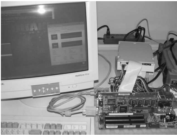
Figure 1: Image of the FPGA-based processor emulator system equipped with standard hardware peripherals, a Xilinx Virtex-4 device in place of a microprocessor chip, all running Windows XP
