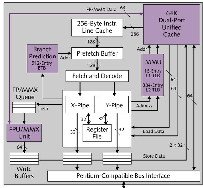
Figure 1. The M2 builds on the 6x86 core with four times as much cache, MMX extensions, a new TLB structure, and a larger BTB.
