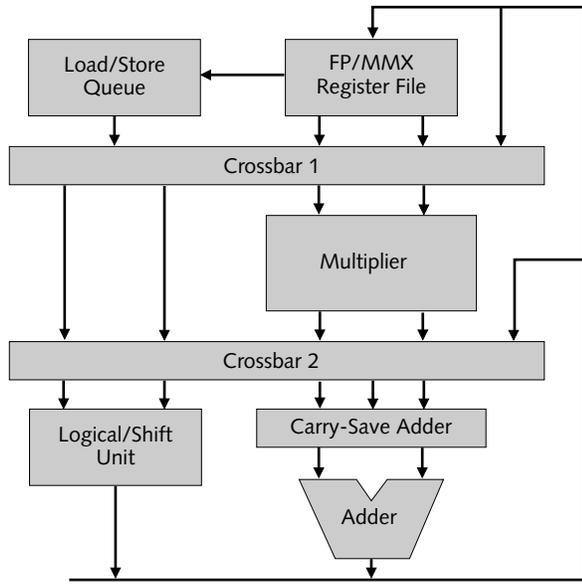
Figure 2. MMX operations are handled by the M2's FPU, which can deliver an MMX multiply-add result every clock cycle.
