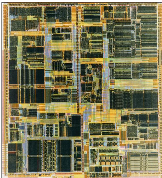
**Figure 4.** Intel's Klamath has 7.5 million transistors and measures 14.9 x 13.7 mm in a 0.28-micron four-layer-metal CMOS process.
