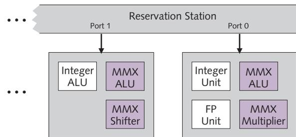
**Figure 3.** A detailed diagram of the two main function units shows that both have an MMX-capable ALU, but only port 0 can accept MMX multiply instructions, and only port 1 can accept MMX shift instructions.
