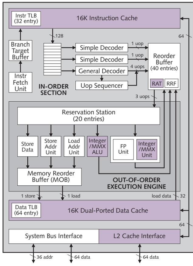
**Figure 2.** This Klamath block diagram shows the significant modifications over Pentium Pro were doubling the on-chip caches and adding MMX functions to both integer units. The register alias table (RAT) now supports renameable segment registers.
