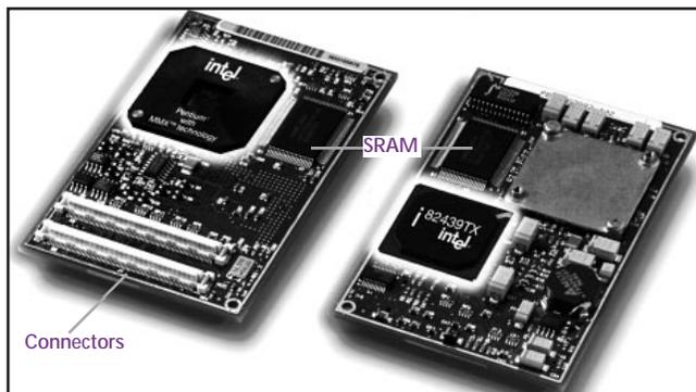
Figure 1. Intel's Mobile Module is a two-sided PC board measuring 2.5" x 4". The bottom (left) shows the footprint of the CPU, one SRAM chip, and the connectors; the top (right) shows the CPU heatsink, the other SRAM, and the 82439TX system-logic chip.
