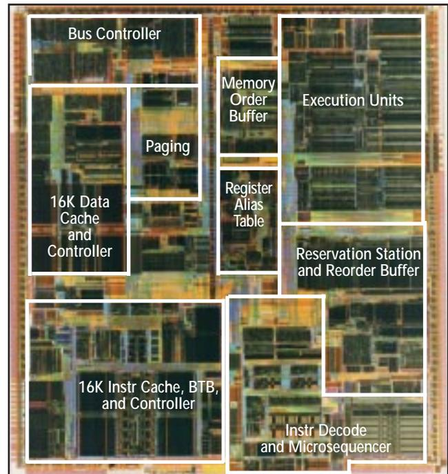
Figure 6. Intel's Pentium II CPU chip has 7.5 million transistors and measures 203 mm<sup>2</sup> when built in Intel's 0.28-micron four-layer-metal CMOS process.
