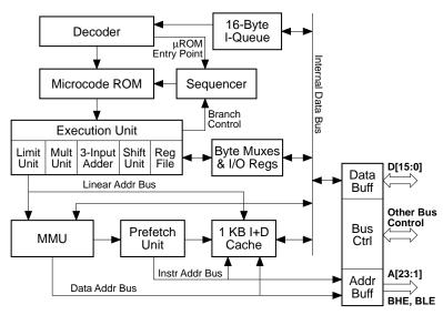
Figure 1. Internal block diagram of the Cyrix 486SLC.
