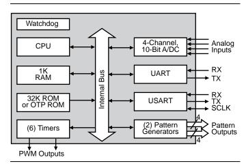
Figure 1. Block diagram of TLCS-900.
