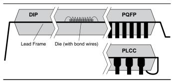
Figure 3. Side view of various plastic packages. Through-hole packages (left) use straight leads, while surface-mount packages (right) have flat leads that either spread out (PQFP) or tuck under the package (PLCC). The center section shows the die bonded to the lead frame and is common among all of these packages.
