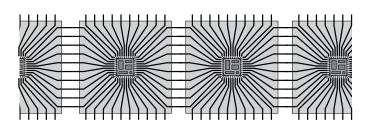
Figure 2. Top view of a set of lead frames with dice wire-bonded in place. These frames are ready to be covered with plastic to form the outer shell of the QFP part.
