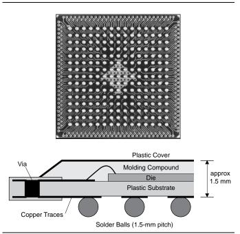
Figure 5. The photograph shows solder balls and traces on the bottom of a ball-grid array (BGA). The diagram shows how signals are routed from the die to the solder balls. (Source: Motorola)
