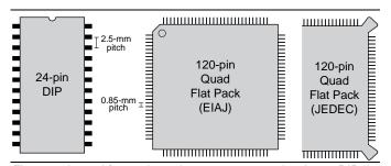
Figure 1. A quad flat pack can have many more pins than a DIP due to its smaller pin spacing. The JEDEC package differs from the EIAJ standard due to its corners. (Parts are approximately actual size.)
