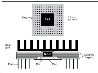
Figure 4. As shown at top, a pin-grid array (PGA) package has several rows of pins on the bottom. The cutaway view (below) shows the die mounted on layers of ceramic.
