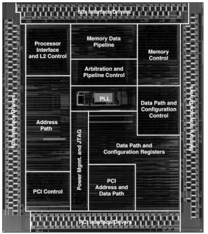
Figure 2. Die photo of the MPC105, which measures  $6.7 \times 5.8$  mm and uses about 300,000 transistors in 0.65-micron CMOS.
