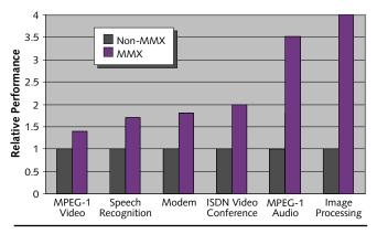
**Figure 1.** MMX improves performance on most multimedia applications by 50–100%, according to simulations of the forthcoming P55C processor. MPEG-1 performance refers to decoding; image processing is pixel manipulation, as in Photoshop. (Source: Intel)
