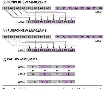
**Figure 3.** (a) Unpack operation converts packed bytes to words with zero extension. (b) PUNPCK can also interleave bytes from two MM registers. (c) Parallel add instruction calculates four 16-bit sums simultaneously.
