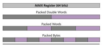
Figure 2. MMX adds three new data types: packed byte, packed word, and packed double word.
