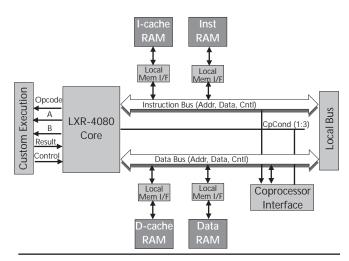
Figure 1. Lexra's LXR-4080 MIPS core includes, at a minimum, the CPU, two caches, and an internal bus interface. The CPU core can be extended either with coprocessors or with custom logic.
