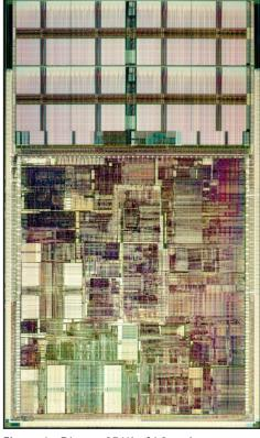
Figure 1. Dixon's 256K of L2 cache consumes 32% of the die, which contains 29 million transistors and measures 10.4 mm  $\times$  17.3 mm in Intel's 0.25-micron five-layer-metal CMOS process. (Source: MDR photoillustration based on Mendocino die photo from Intel)
