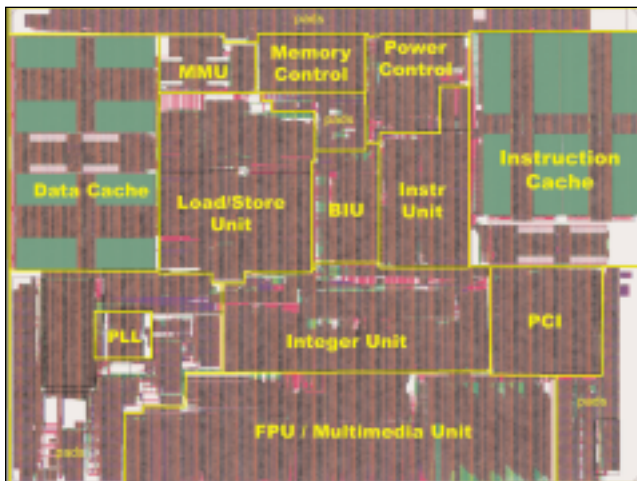
Figure 5. The Crusoe TM3120's die size is 77 mm 2 . Note the PCI controller and memory controller; the north bridge is also on chip.
