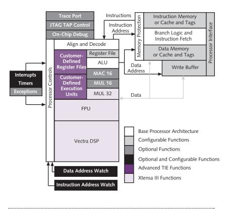
Figure 1. Additions to Tensilica's configurable Xtensa processor core include an FPU, a 32  $\times$  32-bit multiplier, and a vector DSP unit.
