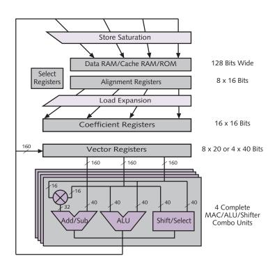
Figure 2. The configurable Vectra DSP unit, shown here in its 16-bit configuration, has four MAC/ALU function units capable of delivering four MACs or eight additions per clock cycle. The MAC/ALU function units connect to registers and memory via four 160-bit buses.
