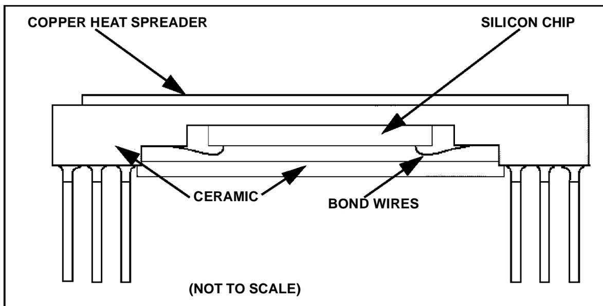
**Figure 1. ST6x86 PGA Package Cross-Sectional View**
