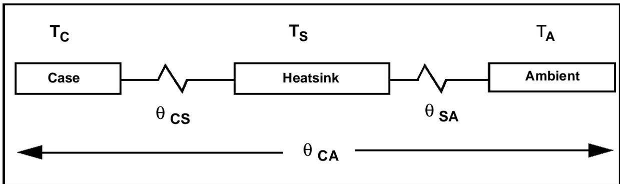
**Figure 2. Thermal Resistor Model for Case to Ambient Thermal Resistance**
