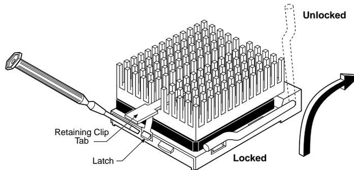
*Figure 4: Removing the CPU Chip*
