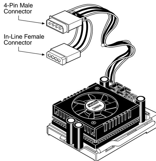
*Figure 7: Attaching the Power Cable*
