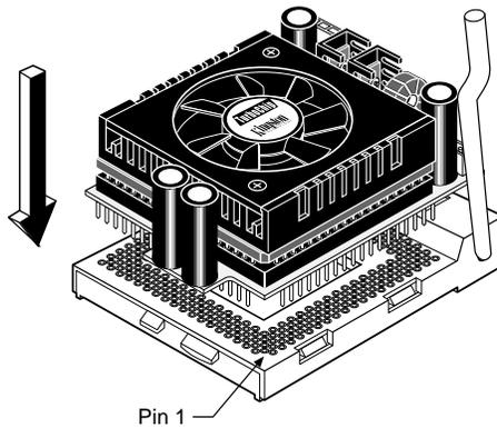
*Figure 5: Orienting the TurboChip*
