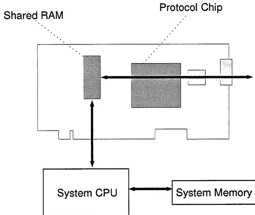
**Figure 1. Shared RAM Adapter.** *The system CPU is involved in the transfer of each and every byte of every frame.*
