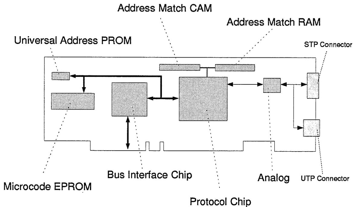
**Figure 4. IBM Token-Ring LANStreamer MC 32 Adapter.** *Anatomy of an adapter.*
