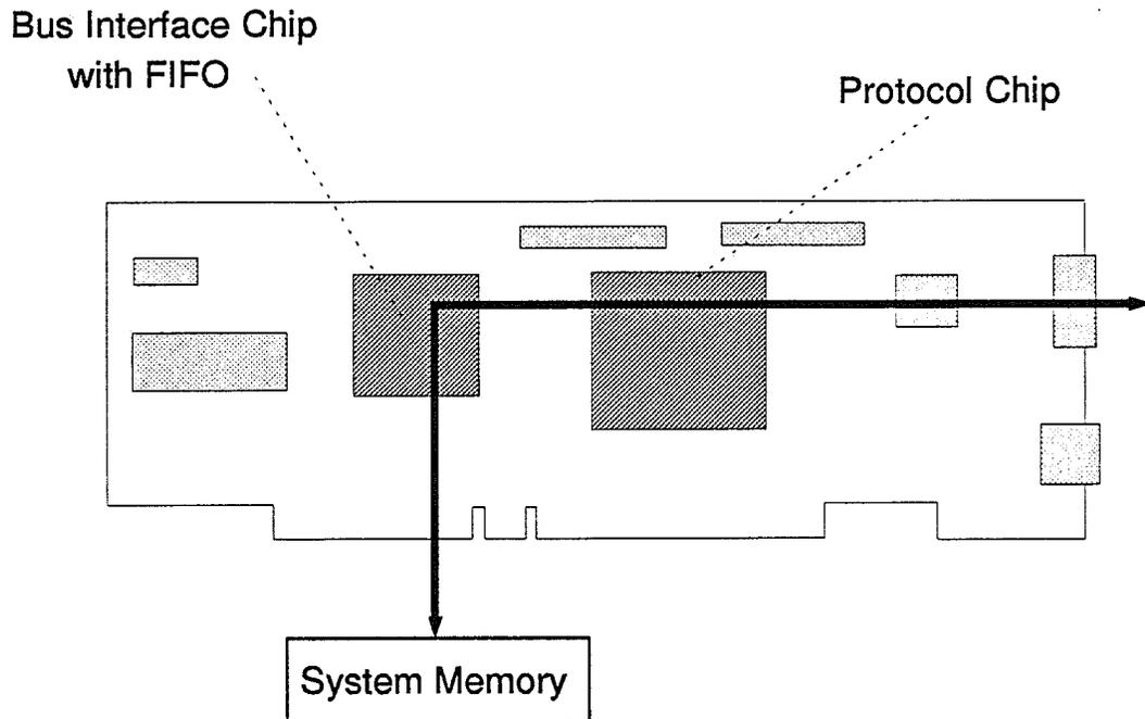
**Figure 3. LANStreamer Adapter.** *The adapter has no buffer memory. Frames are transferred directly between the LAN and system memory.*
