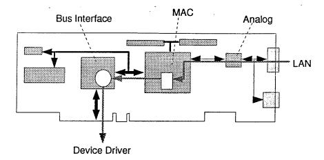
Provides a way for the microcode to deliver MAC frames and Ring Status to the system.
