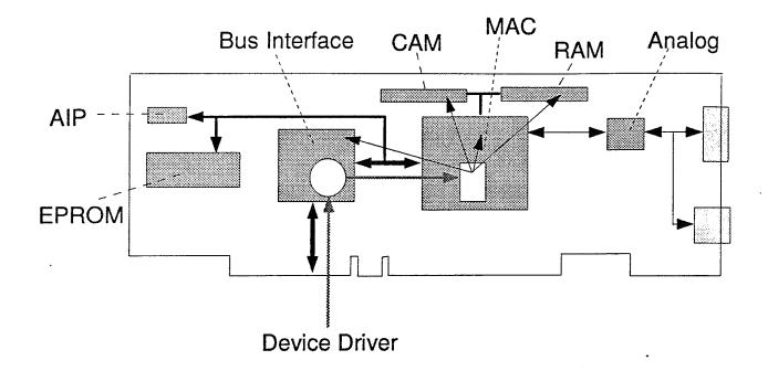
Device Driver places SRB in Common RAM via LAP Interface.
