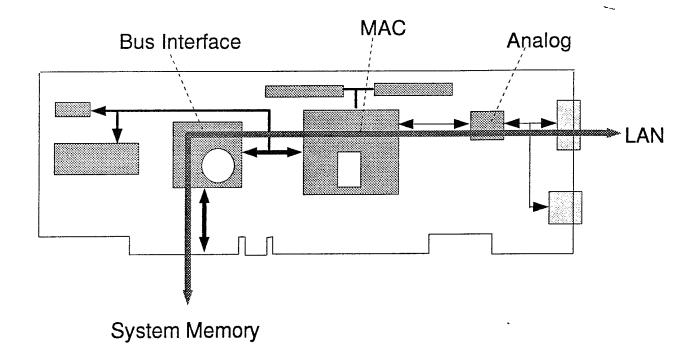
LLC Frames are Transmitted and Received via DMA Channel.
