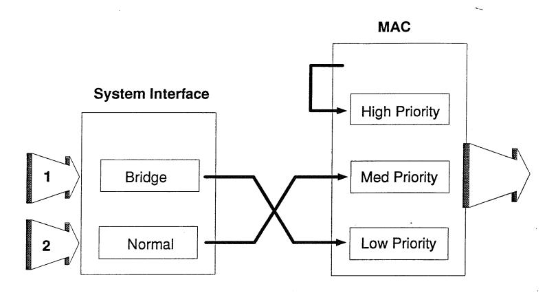
System Interface Channel 1 is used for bridge forwarding traffic.
