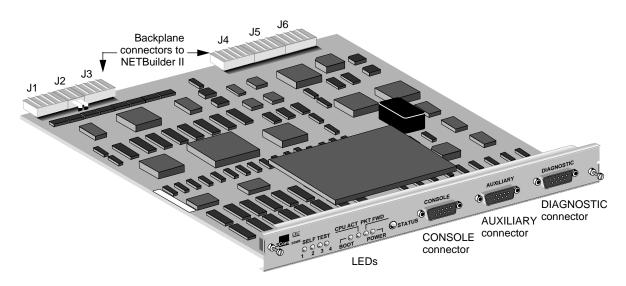
**LEDs** The nine LEDs display the diagnostic and operational activity of the NETBuilder II Bridge/Router. Table 2-2 lists each of the LEDs and their functions.
