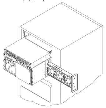
**Replacement:** Replace in reverse order. Ensure that the retained screws are properly engaged, as they draw the fan assembly into the fan connectors.
