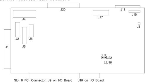
J2 Serial port connector to inside bulkhead card J3 Speaker connector J4 Diskette drive connector J5 Parallel Port connector J6 Keyboard/mouse connector to inside bulkhead card Write protect DASD FLASH (if jumper is on pins) J16 J17 Control panel connector from System Rack. J18 Test Port 0 Test Port 1 J19 J20 Test Port 2 **J22** Write protect boot FLASH (if jumper is set between pins 2 and 3)
