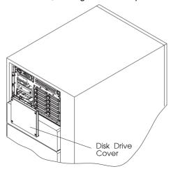
3. Each hot swap disk drive you plan to replace must have the hot swap SCSI disk drive carrier attached.
