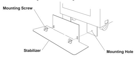
8. Use the crank supplied with the system unit to alternately tighten the mounting screws until they are firmly seated.
