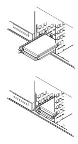
e. Move the carrier latch to the locked position. If the carrier does not lock, check that the drive carrier is fully seated in the backplane. When the drive carrier is fully seated and power is turned on, the green LED on the drive carrier is illuminated.
