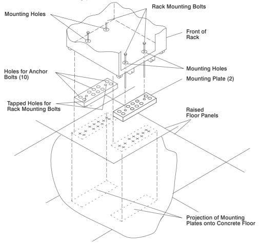
9. At the marked location of the tapped mounting holes, drill two holes approximately 1 inch to allow clearance for the ends of the two rack-mounting bolts (the
