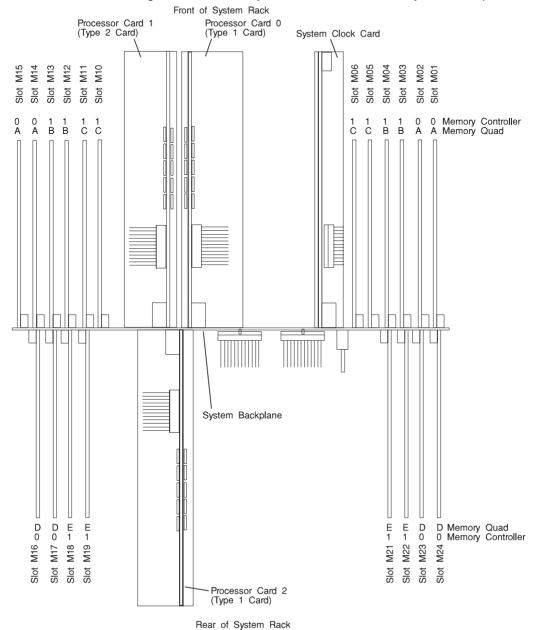
R1 Memory Cards are the primary memory cards used in the S70. All S70 memory cards are installed in four card functional units called quads. The quads must be composed of the four cards of the same type. The complete set of four cards must be properly installed in the proper card slots for the newly installed memory to work. See the figure on page 1-20 for the location of the card slots that are in each quad.
