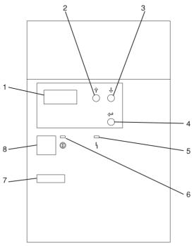
Operator Panel Display 1 Scroll Up Pushbutton 2 Scroll Down Pushbutton 3 4 **Enter Pushbutton** 5 Attention LED 6 Power On LED 7 Serial Number 8 Power Pushbutton
