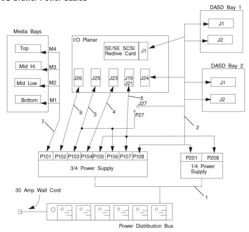
**Note:** The power distribution bus, and the Y-cable (index number 1) shown above are not used on -48 V dc systems. See "Input/output Rack -48 Volt Power Distribution Assembly (2 of 2)" on page 10-56 for -48 V dc power distribution parts.
