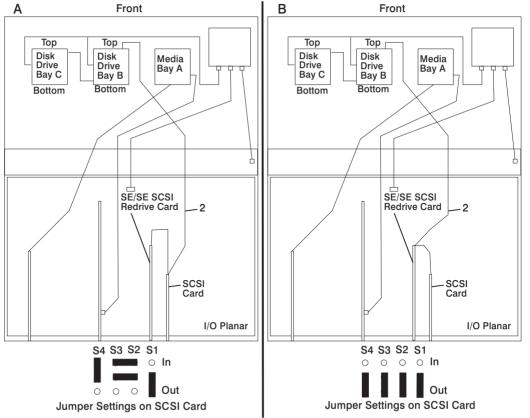
Figure A shows SCSI disk drive bay cabling and SCSI card jumper settings when using cable FRU PN 93H2456 Figure B shows SCSI disk drive bay cabling and SCSI card jumper settings when using cable FRU PN 07L7005
