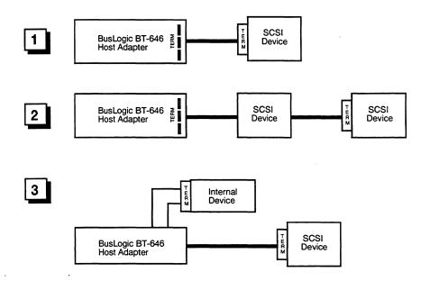
Figure 2-2. SCSI Terminator Configurations
