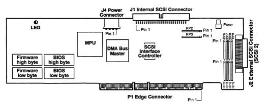
Figure 2-1. The BT-646 Host Adapter Board
