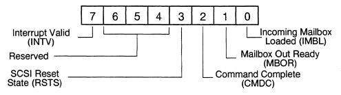
Figure 4-5. Interrupt Register (Read Only)
