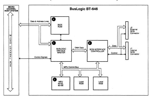
Figure 1-2. Host Adapter Architecture
