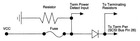
Figure 3-2. Terminator Power Schematic
