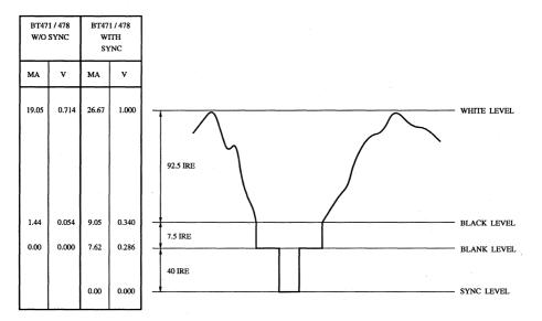
*Note:* 75  $\Omega$  doubly-terminated load and SETUP = 7.5 IRE. VREF = 1.235 V and RSET = 147  $\Omega$ . RS-343A levels and tolerances are assumed on all levels.
