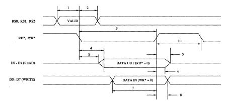
Figure 7. MPU Read/Write Timing Dimensions.
