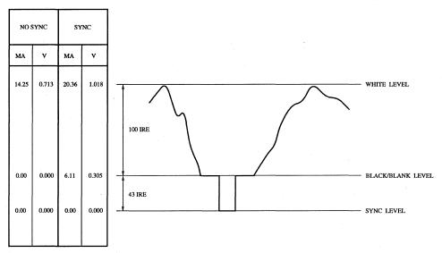
*Note:* 50  $\Omega$  load and SETUP = 0 IRE. VREF = 1.235 V and RSET = 182  $\Omega$ . PS/2 levels and tolerances are assumed on all levels.
