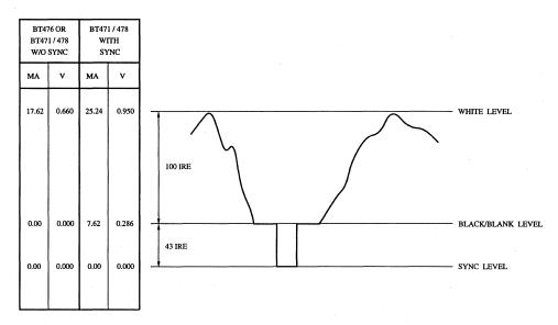
*Note:* 75  $\Omega$  doubly-terminated load and SETUP = 0 IRE. VREF = 1.235 V and RSET = 147  $\Omega$ . RS-343A levels and tolerances are assumed on all levels.
