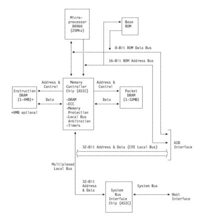
Figure 2-1. Co-Processor Platform Block Diagram
