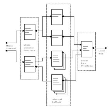
All data transactions, including Bus Master transfers, are subject to intermediate buffering. A diagram of this intermediate buffering is shown in Figure 8-1.
