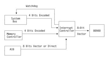
Figure 6-1 shows the interrupt flow on the co-processor platform.
