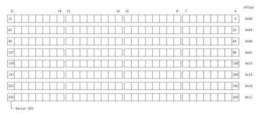
When an interrupt service routine is invoked, it sets the bit corresponding to the vector number of interrupt being serviced.
