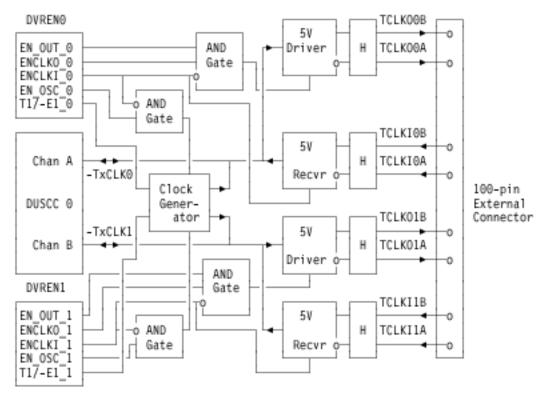
Figure 13-10. TxCLK Block Diagram
