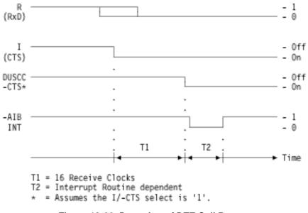
Figure 13-22. Detection of DTE Call Request
