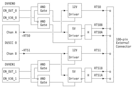
Figure 13-12. RTS Block Diagram
