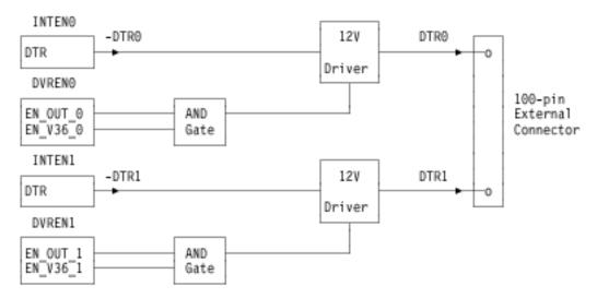
Figure 13-14. DTR Block Diagram
