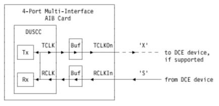
Figure 13-33. X.21 DTE Operation
