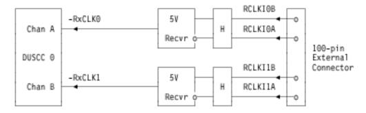
Figure 13-11. RxCLK Block Diagram
