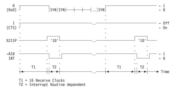
Figure 13-20. Detection of DCE Connection in Progress
