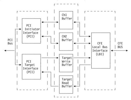
Figure 9-1. PCI Bus Intermediate Buffering
