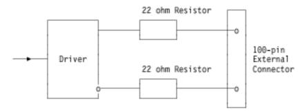
Figure 13-6. Homologation Circuit for Balanced Drivers
