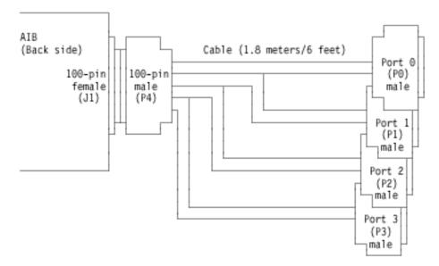
Figure 13-25. AIB Cable Assembly
