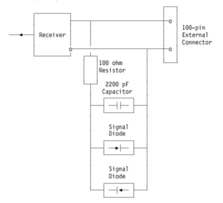
Every balanced receiver has the line impedance circuitry illustrated in Figure 13-6 to satisfy the homologation specifications.
