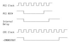
Figure 2-2. Reset Delay Timing
