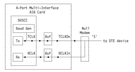
Figure 13-34. X.21 DCE Operation — Low Speed
