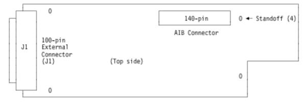
Figure 13-2. Card Layout of the 4-Port Multi-Interface AIB—Top Side
