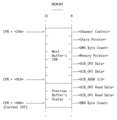
terminal count or the end-of-process interrupts. In theory, this list of buffers could occupy any amount of free memory. This concept is detailed in Figure 13-4.
