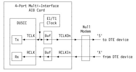
Figure 13-35. X.21 DCE Operation — High Speed
