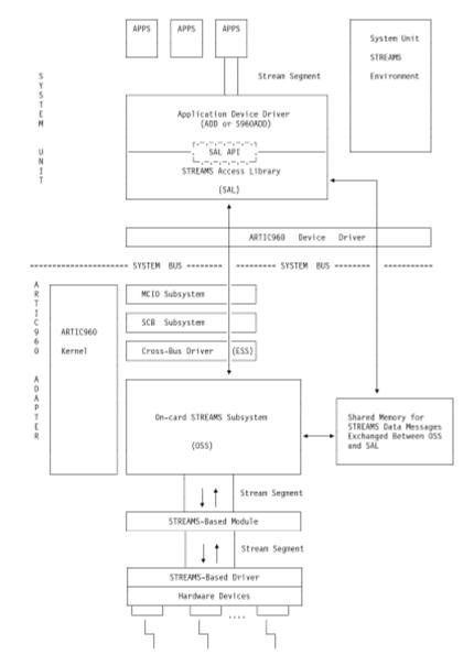
Figure 1-1. System Unit and Co-Processor Components
