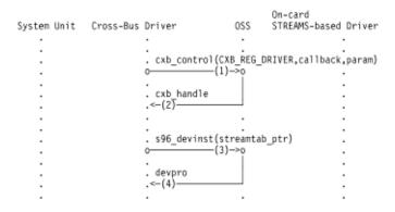
Figure 5-2. Registering a Cross-bus Driver with OSS
