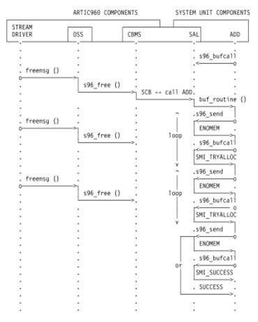
Figure 7-1. Downstream Flow — SMI\_TRYALLOC Situations
