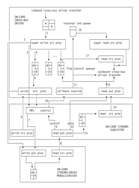
Figure 5-1. Example of an On-card Lower-end Interface
