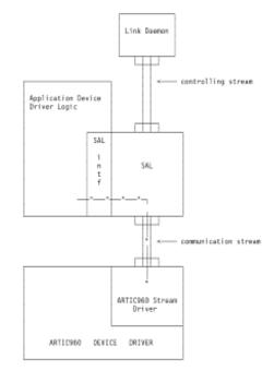
Figure 6-1. AIX Application Device Driver Communication with RadiSys ARTIC960 Adapter Application Device Driver
