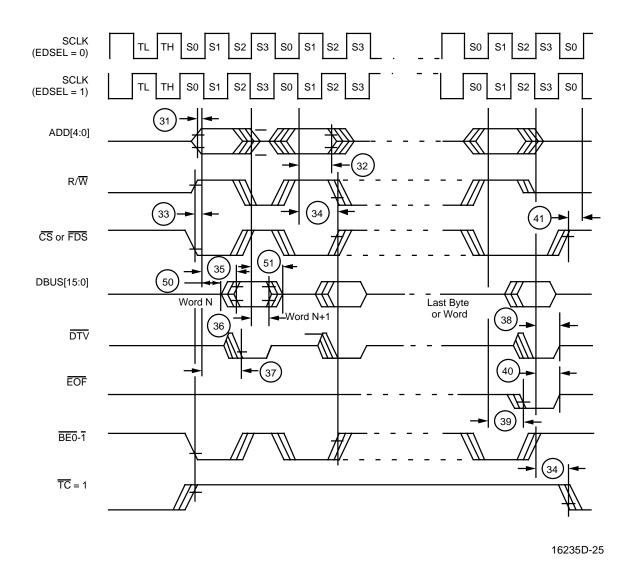
Host System Interface—2-Cycle Receive FIFO/Register Read Timing
