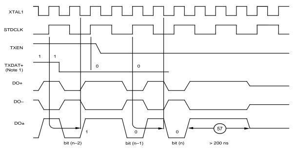
Note: TXDAT+ is the internal version of the signal, and is shown for clarification only.
