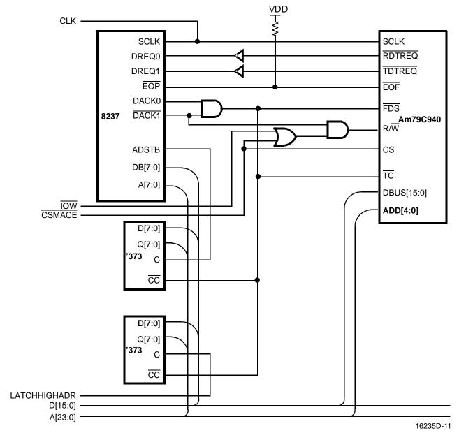
**System Interface - Motherboard DMA Example**
