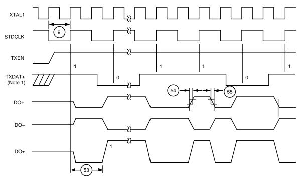
Note: TXDAT+ is the internal version of the signal, and is shown for clarification only.
