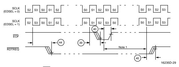
**Note:** Once the host detects the  $\overline{\text{EOF}}$  output active from the MACE device (S2/S3 edge), if no other receive packet exists in the RCVFIFO which meets the assert conditions for  $\overline{\text{RDTREQ}}$ , the MACE device will deassert  $\overline{\text{RDTREQ}}$  within 4 SCLK cycles (S0/S1 edge). This is consistent for both 2 or 3 cycle read operations.
