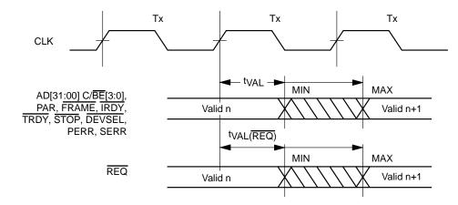
Figure 65. Output Valid Delay Timing
