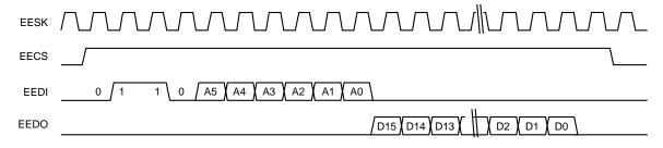
Figure 67. EEPROM Read Functional Timing
