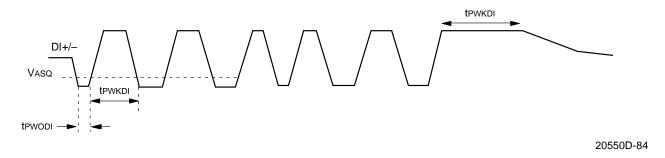
Figure 81. Receive Timing
