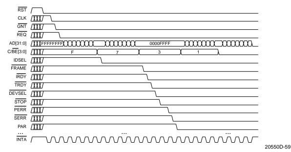
Figure 56. NAND Tree Waveform
