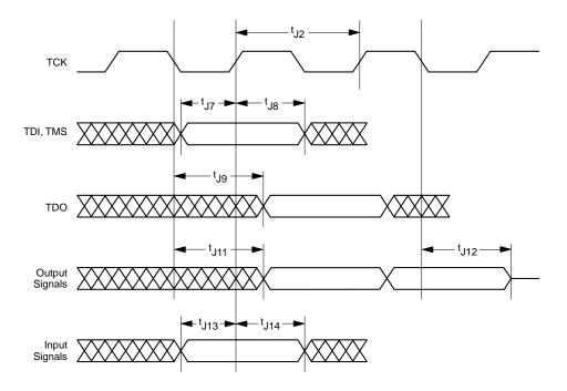
Figure 70. JTAG (IEEE 1149.1) Test Signal Timing
