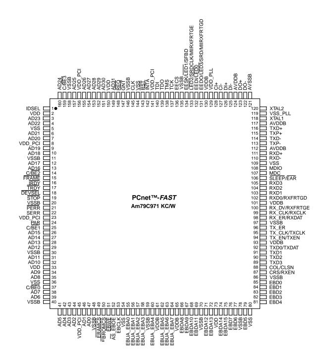
Pin 1 is marked for orientation.
