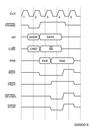
Figure 6. Disconnect Of Slave Cycle When Busy
