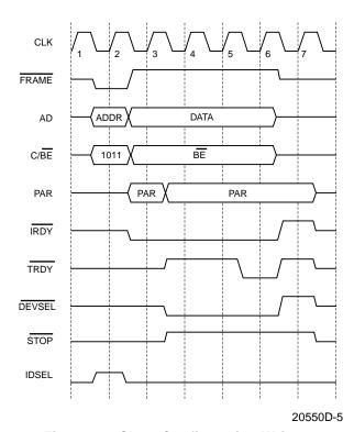
Figure 2. Slave Configuration Write
