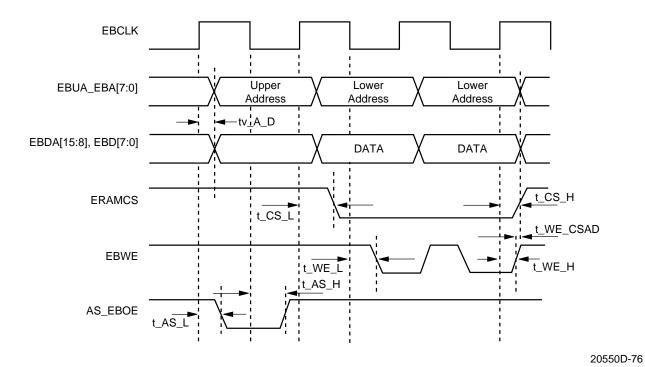
Figure 73. Expansion Bus SRAM Write Timing--Normal SRAM Operation
