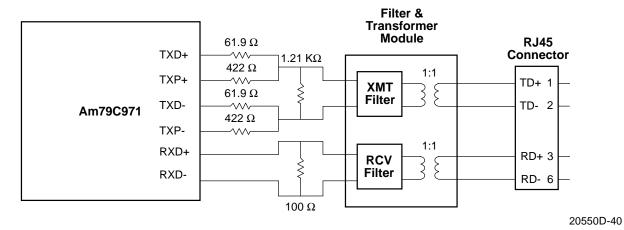
Figure 37. 10BASE-T Interface Connection
