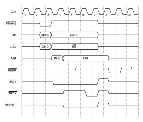
Figure 10. Slave Cycle Data Parity Error Response
