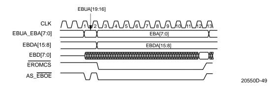
Figure 46. Flash Read from Expansion Bus Data Port
