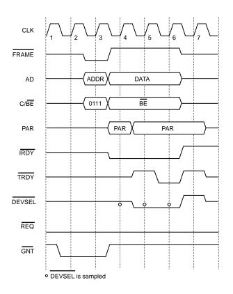
Figure 19. Preemption During Non-Burst Transaction
