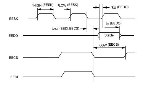
Figure 68. Automatic PREAD EEPROM Timing
