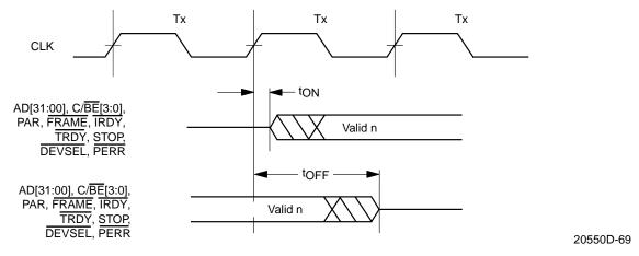
Figure 66. Output Tri-state Delay Timing
