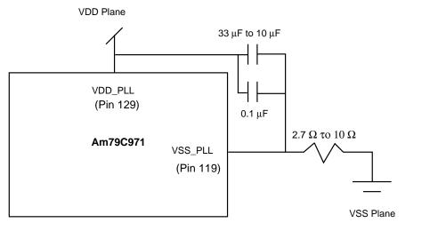
Figure 2. Power and Ground Pin Connections
