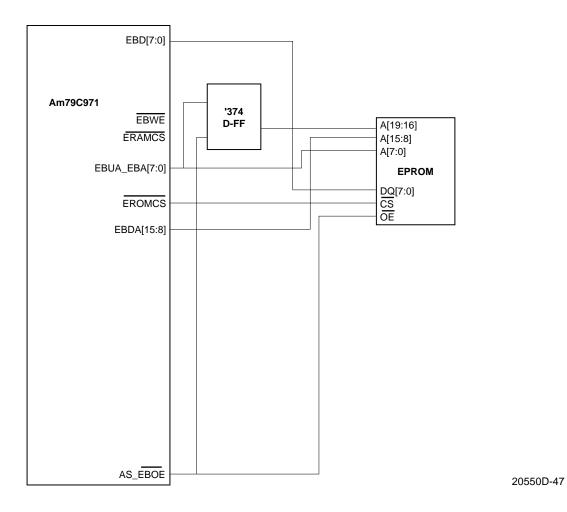
Figure 44. EPROM Only Configuration for the Expansion Bus (>64K EPROM)
