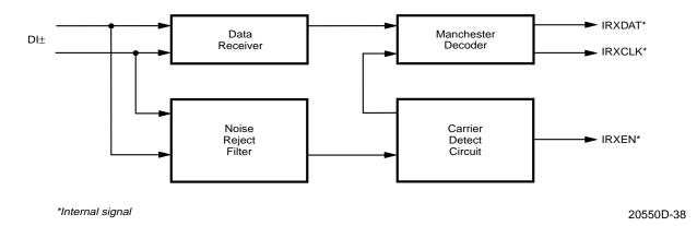
Figure 35. Receiver Block Diagram
