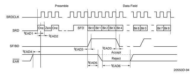
Figure 91. Reject Timing
