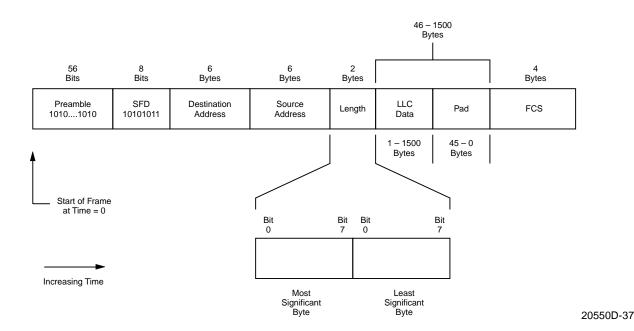
Figure 34. IEEE 802.3 Frame And Length Field Transmission Order
