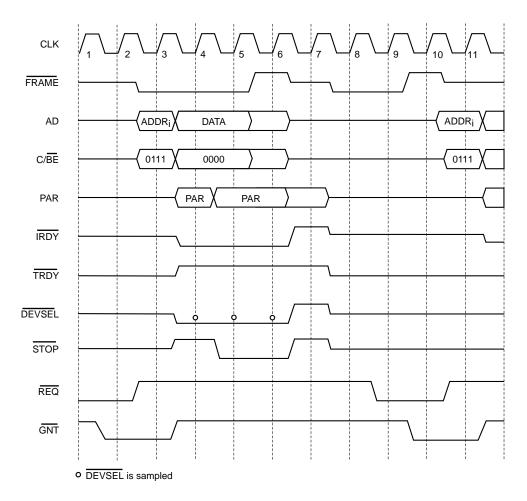
Figure 17. Disconnect Without Data Transfer
