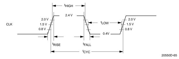
Figure 62. CLK Waveform for 5 V Signaling
