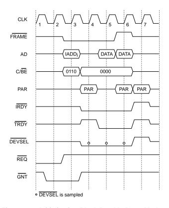
Figure 24. Initialization Block Read In Burst Mode
