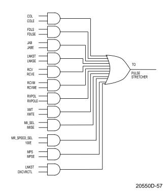
Figure 54. LED Control Logic
