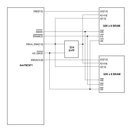
Figure 48. SRAM Only Configuration for the Expansion Bus
