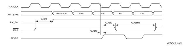
Figure 92. Reject Timing - External PHY MII @ 25 MHz
