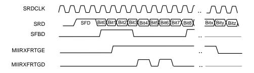
Figure 41. Internal PHY Receive Frame Tagging
