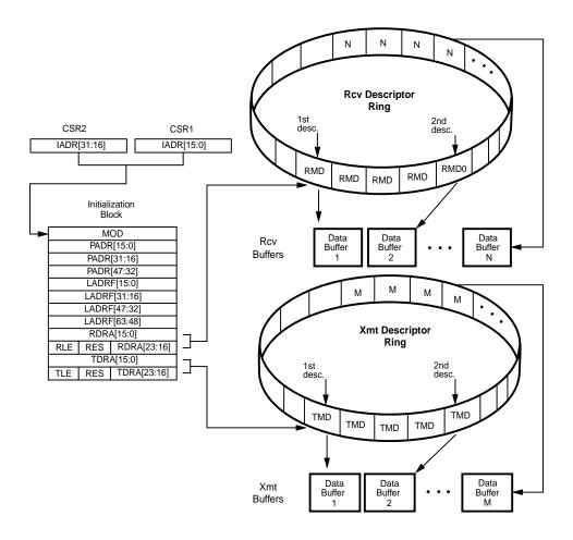
Figure 31. 16-Bit Software Model
