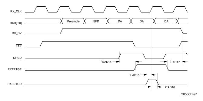
Figure 94. Receive Frame Tag Timing with Media Independent Interface
