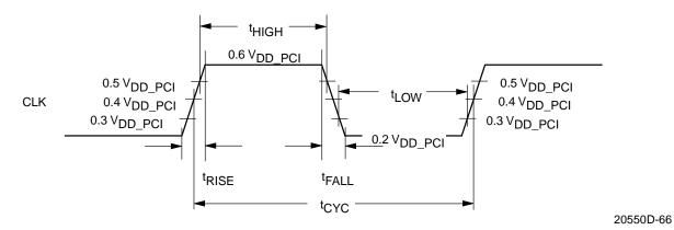
Figure 63. CLK Waveform for 3.3 V Signaling
