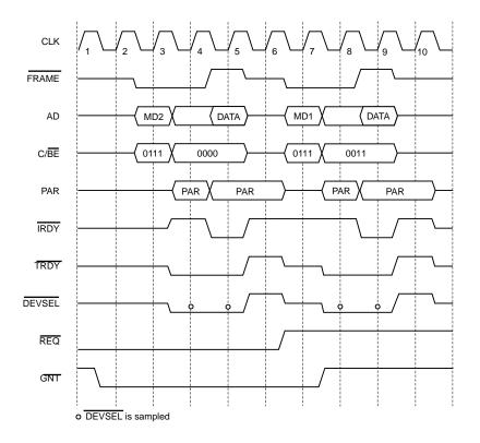
Figure 27. Descriptor Ring Write In Non-Burst Mode
