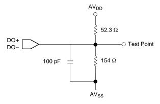
Figure 59. AUI DO Switching Test Circuit
