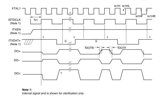
Figure 78. Transmit Timing - Start of Frame
