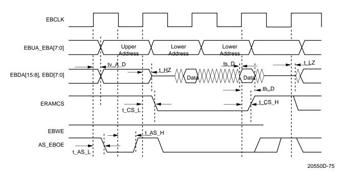
Figure 72. Expansion Bus SRAM Read Timing--Normal SRAM Operation
