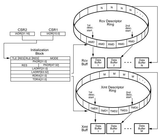
Figure 32. 32-Bit Software Model
