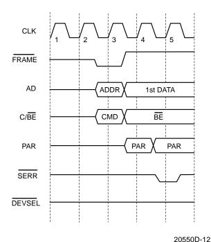
Figure 9. Address Parity Error Response
