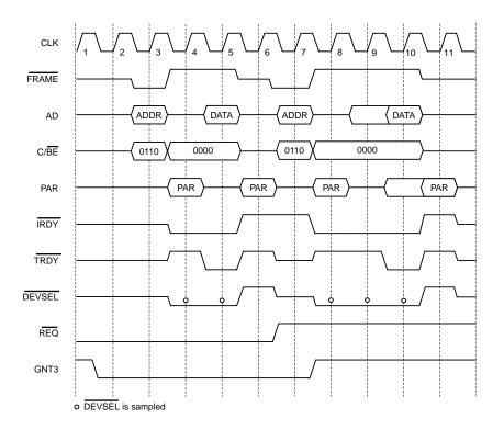
Figure 12. Non-Burst Read Transfer
