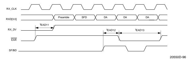
Figure 93. Reject Timing - External PHY MII @ 2.5 MHz
