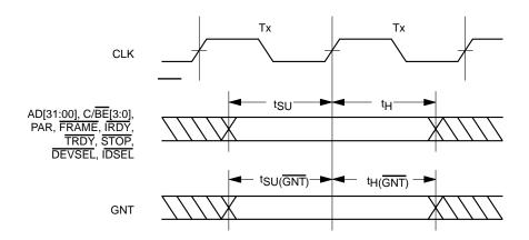
Figure 64. Input Setup and Hold Timing
