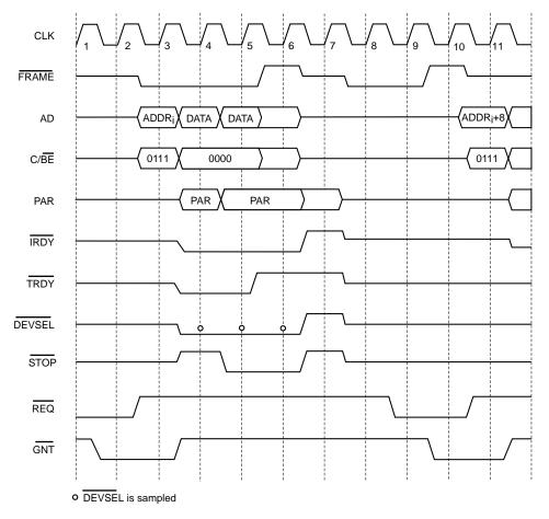
Figure 16. Disconnect With Data Transfer
