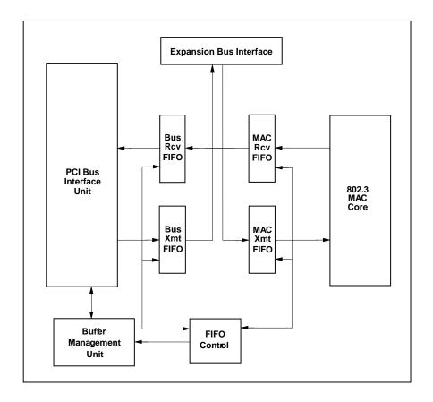
Figure 51. Block Diagram Low Latency Receive Configuration
