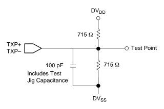
Figure 61. TXP Outputs Test Circuit
