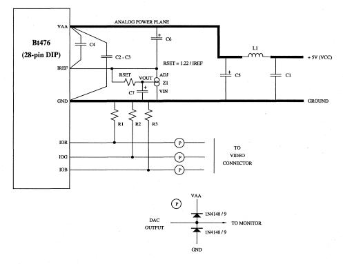
Note: Each set of VAA and GND pins must be separately decoupled.
