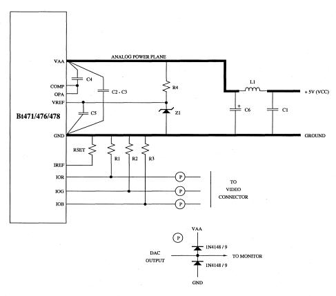
Note: Each set of VAA and GND pins must be separately decoupled.
