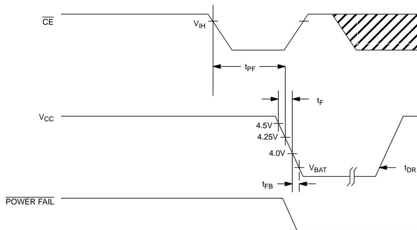
**POWER-UP POWER-DOWN TIMING** $(t_A = 25^\circ\text{C})$
