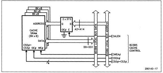
Figure 4-4A. Direct Mapped Cache without Data Buffers
