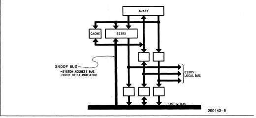
Figure 1-4. 82385 Bus Watching—Monitor System Bus Write Cycles
