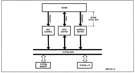
Figure 1-1. 80386 System Bus Structure
