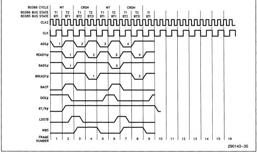
Figure 5-3G. Interleaved WT/CRDH Cycles—(N = 1)
