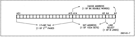
Figure 2-2. 80386 Address Bus Bit Fields—Direct Mapped Organization
