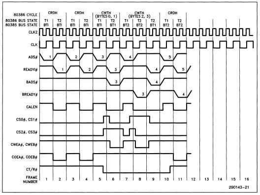
Figure 4-5A. Cache Read and Write Cycles—Direct Mapped (N = 1)
