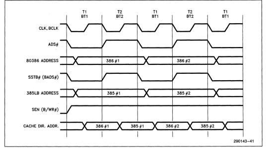
Figure 5.4. Interleaved Snoop and 80386 Accesses to the Cache Directory
