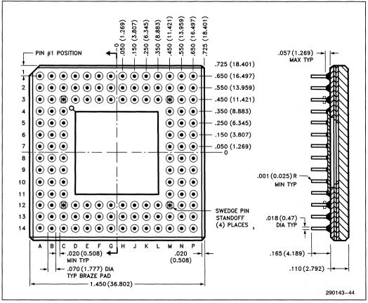
Figure 8-3. 132-Pin PGA Package Dimensions
