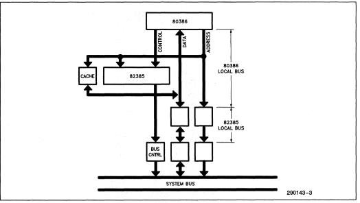
Figure 1-2. 80386/82385 System Bus Structure
