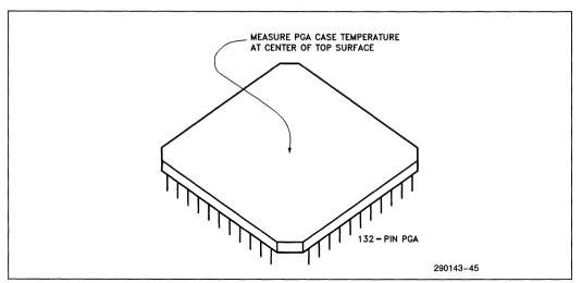
Figure 8-4. Measuring 82385 PGA Case Temperature
