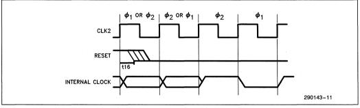
Figure 3-2. Reset/Internal Phase Relationship
