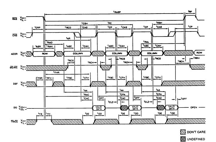
NOTE: 1. WRITE cycles or READ-MODIFY-WRITE cycles may be mixed with READ cycles while in FAST PAGE MODE.
