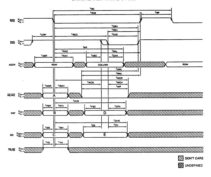
NOTE: 1. The logic states of "A", "B", "C", "D" and "E" determine the type of WRITE operation performed. See the Write Cycle Function Table for a detailed description.
