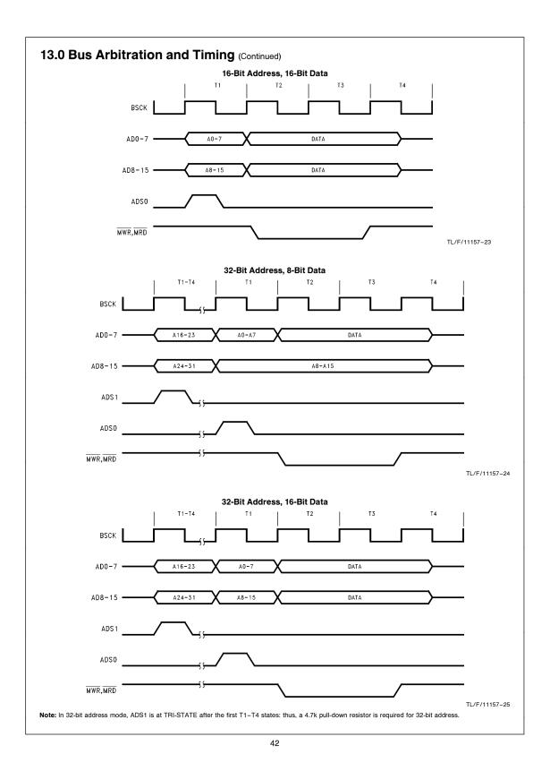
When in 32-bit mode four additional BSCK cycles are required per burst. The first bus cycle (T1'-T4') of each burst is used to output the upper 16-bit addresses. This 16-bit address is programmed in RSAR0 and RSAR1 and points to a 64k page of system memory. All transmitted or received packets are constrained to reside within this 64k page.
