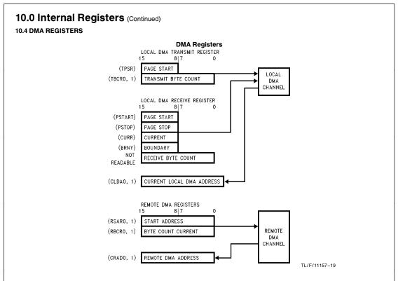
The DMA Registers are partitioned into groups; Transmit, Receive and Remote DMA Registers. The Transmit registers are used to initialize the Local DMA Channel for transmission of packets while the Receive Registers are used to initialize the Local DMA Channel for packet Reception. The Page Stop, Page Start, Current and Boundary Registers are used by the Buffer Management Logic to supervise the Receive Buffer Ring. The Remote DMA Registers are used to initialize the Remote DMA.
