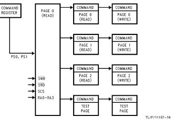
10.2 REGISTER ADDRESS ASSIGNMENTS Page 0 Address Assignments (PS1 = 0, PS0 = 0)
