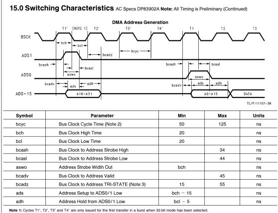
Note 2: The rate of bus clock must be high enough to support transfers to/from the FIFO at a rate greater than the serial network transfers from/to the FIFO. Note 3: These limits include the RC delay inherent in our test method. These signals typically turn off within 15 ns, enabling other devices to drive these lines with no contention.
