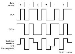
The signal with pre-emphasis shown above is generated by resistively combining TXO+ and TXOd-. This signal along with its complement is passed to the transmit filter.
