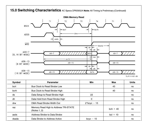
Note 1: During a burst A8-A15 are not TRI-STATE if byte wide transfers are selected. On the last transfer A8-A15 are TRI-STATE as shown above. Note 2: These limits include the RC delay inherent in our test method. These signals typically turn off within bch + 15 ns, enabling other devices to drive these lines with no contention.
