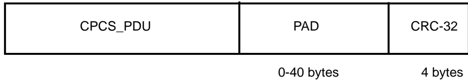
Figure 1-5. TranSwitch Proprietary CRC-32
