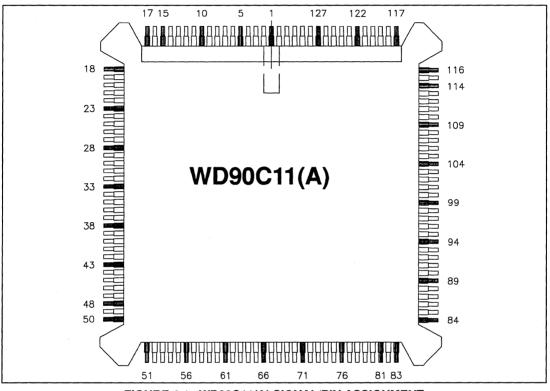
FIGURE 4-1. WD90C11(A) SIGNAL/PIN ASSIGNMENT
