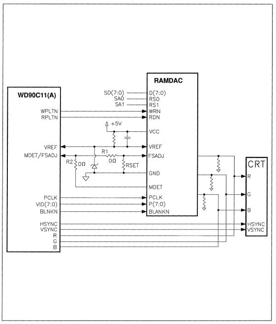
FIGURE A-7. WD90C11(A) WITH RAMDAC INTERFACE
