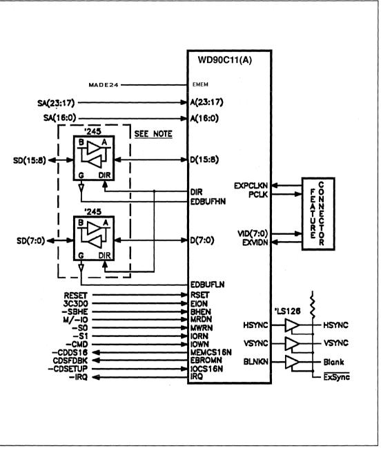
FIGURE A-6. 16-BIT MICRO CHANNEL INTERFACE
