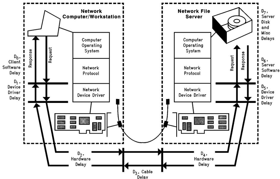
**FIGURE 2. Representation of System Delays that Impact Performance**
