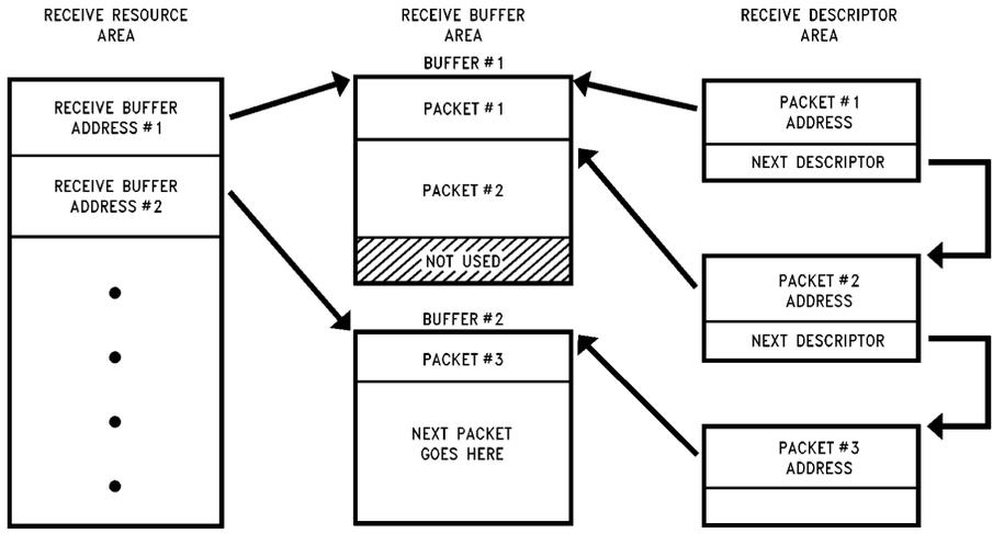
FIGURE 14. Linked List Packet Receive Buffer Structure
