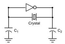
a. Inverting Amplifier Configuration
