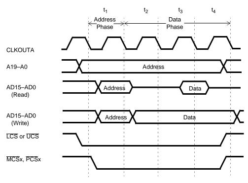
Figure 3-2 Am186EM Microcontroller—Read and Write with Address Bus Disable In Effect
