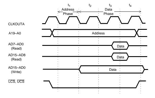
Figure 3-3 Am188EM Microcontroller Address Bus—Normal Read and Write Operation
