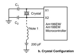
Note 1: Use for Third Overtone Mode XTAL Frequency L1 Value (Max 20 MHz  $12 \mu H \pm 20\%$   $8.2 \mu H \pm 20\%$  33 MHz  $4.7 \mu H \pm 20\%$
