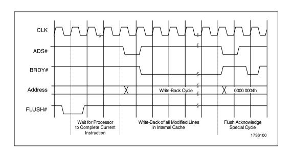
Figure 3-16. Cache Invalidation Using FLUSH#
