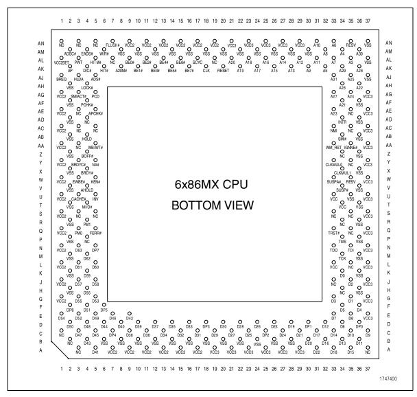
Figure 5-2. 296-Pin SPGA Package Pin Assignments (Bottom View)
