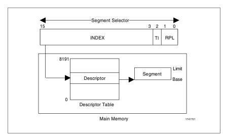
Figure 2-3. Segment Selector in Protected Mode
