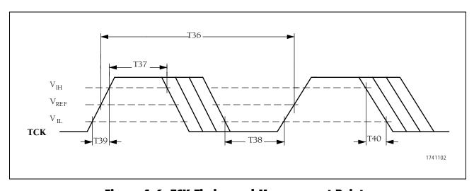
Figure 4-6. TCK Timing and Measurement Points
