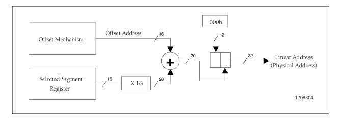
Figure 2-26. Real Mode Address Calculation
