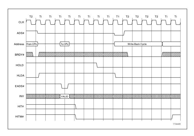
Figure 3-22. HOLD Inquiry Cycle that Hits on a Modified Line
