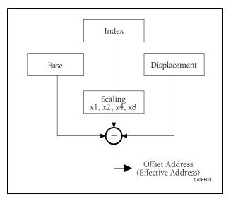
Figure 2-25. Offset Address Calculation
