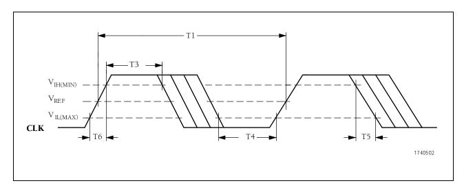
Figure 4-2. CLK Timing and Measurement Points
