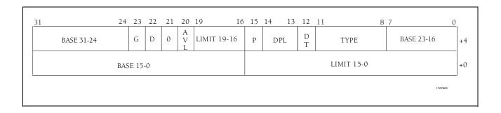
Figure 2-8. Application and System Segment Descriptors
