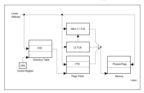
Figure 1-3. Paging Mechanism within the Memory Management Unit
