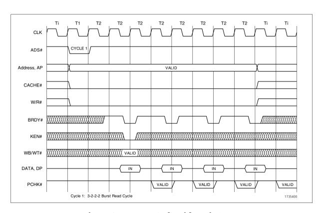
Figure 3-7. Burst Cycle with Wait States
