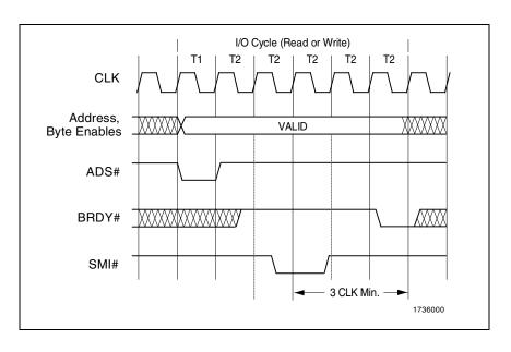
Figure 3-15. SMM I/O Trap Timing
