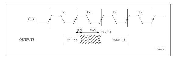
Figure 4-3. Output Valid Delay Timing
