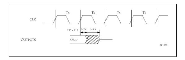
Figure 4-4. Output Float Delay Timing
