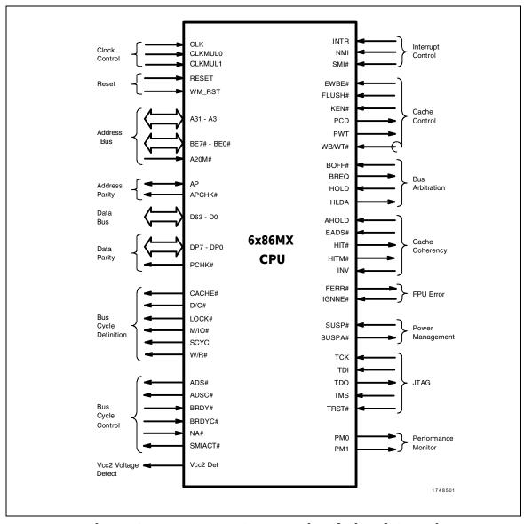
Figure 3-1. 6x86MX CPU Functional Signal Groupings
