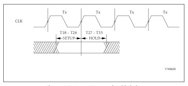
Figure 4-5. Input Setup and Hold Timing
