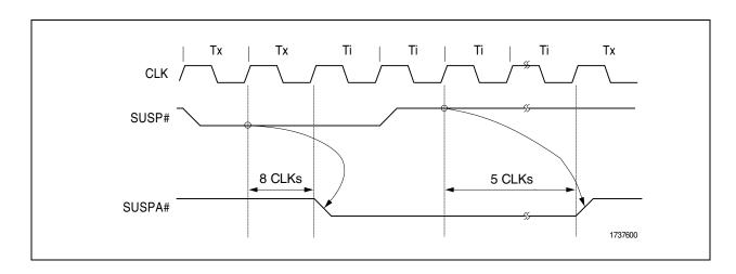
Figure 3-31. SUSP# Initiated Suspend Mode
