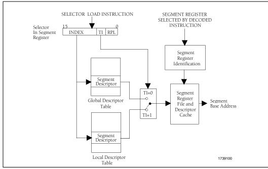
Figure 2-28. Selector Mechanism PRELIMINARY
