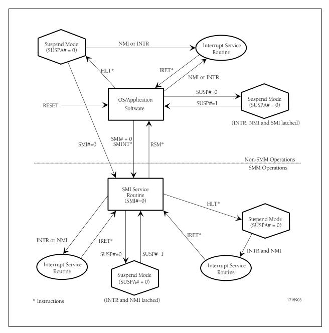
Figure 2-39. SMM and Suspend Mode State Diagram
