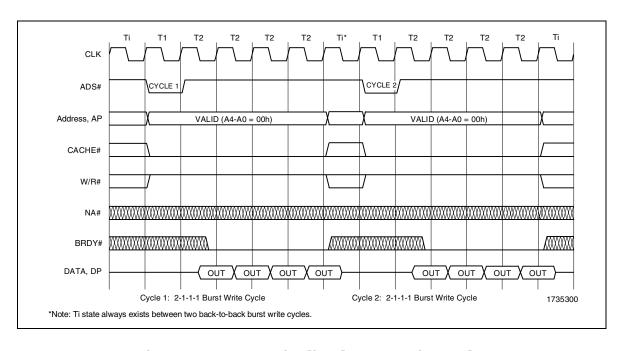
Figure 3-9. Non-Pipelined Burst Write Cycles
