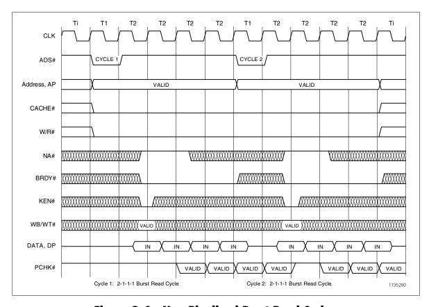
Figure 3-6. Non-Pipelined Burst Read Cycles
