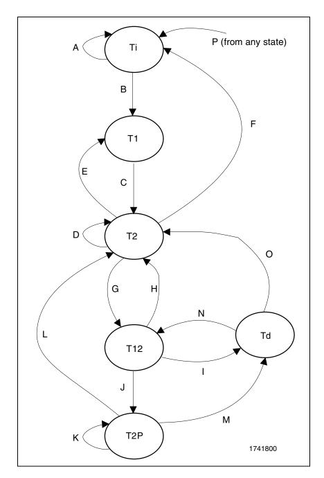
Figure 3-3. 6x86MX CPU Bus State Diagram
