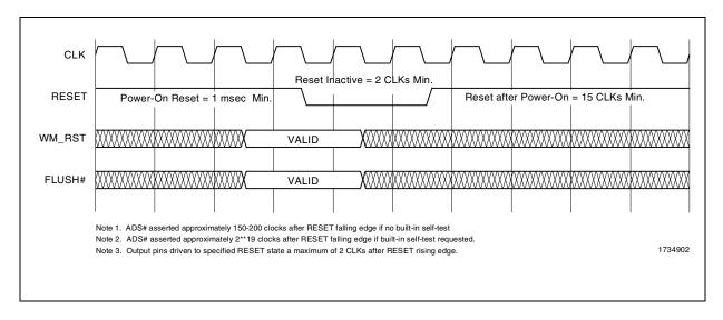
Figure 3-2. RESET Timing
