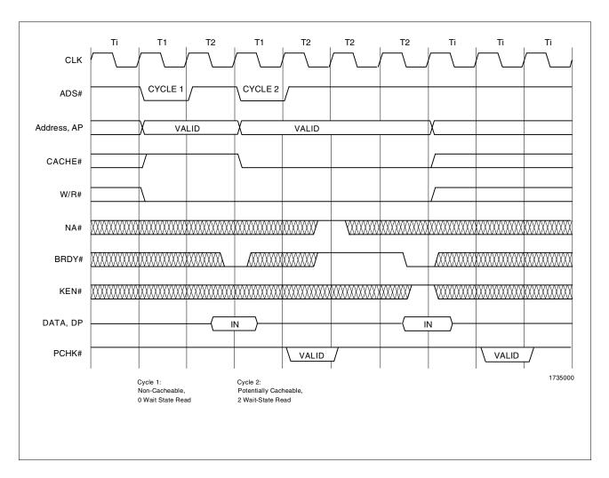
Figure 3-4. Non-Pipelined Single Transfer Read Cycles
