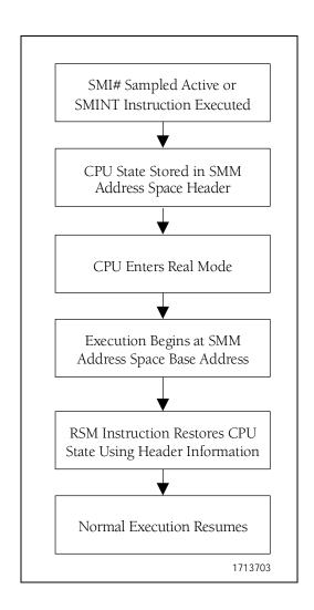
Figure 2-35. SMI Execution Flow Diagram
