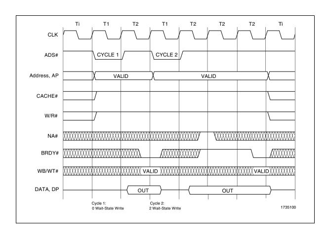
Figure 3-5. Non-Pipelined Single Transfer Write Cycles
