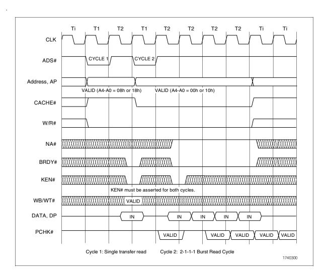
Figure 3-8. "1+4" Burst Read Cycle
