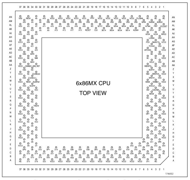
Figure 5-1. 296-Pin SPGA Package Pin Assignments
