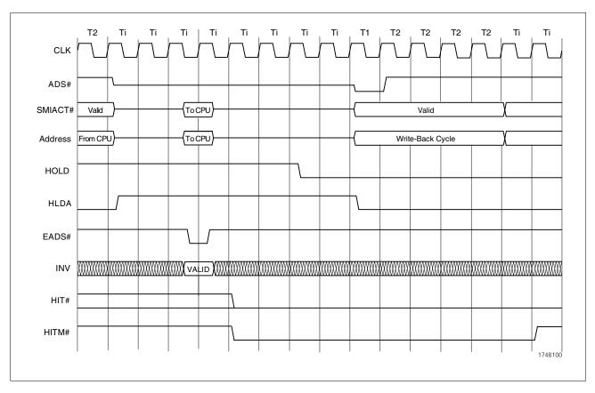
Figure 3-27. Hold Inquiry that Hits on a Modified Data Line
