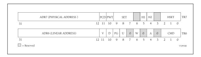
Figure 2-31. TLB Test Registers
