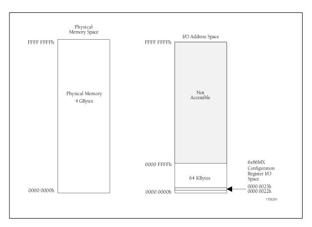
Figure 2-24. Memory and I/O Address Spaces
