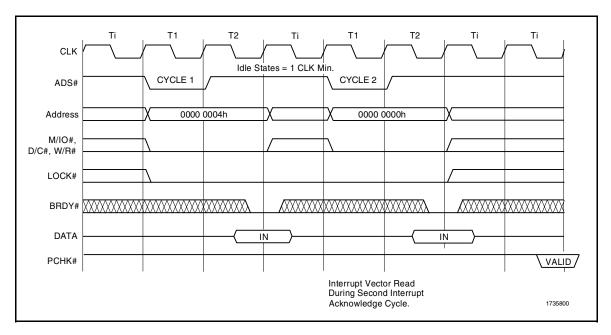
Figure 3-13. Interrupt Acknowledge Cycles
