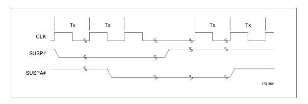
Figure 3-33. Stopping CLK During Suspend Mode
