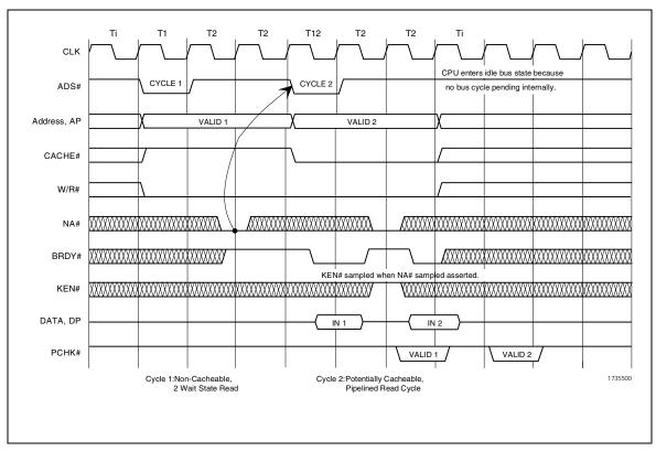
Figure 3-10. Pipelined Single Transfer Read Cycles
