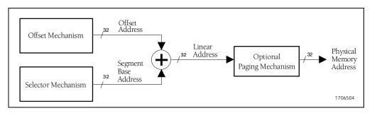
Figure 2-27. Protected Mode Address Calculation
