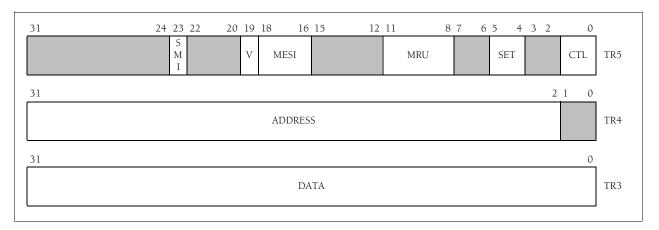
Figure 2-33. Cache Test Registers
