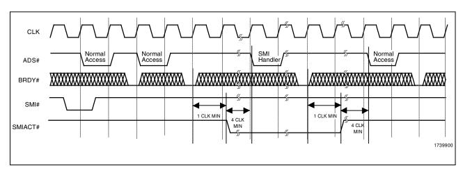
Figure 3-14. SMIACT# Timing in SL Compatible Mode
