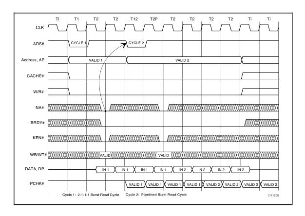
Figure 3-11. Pipelined Burst Read Cycles
