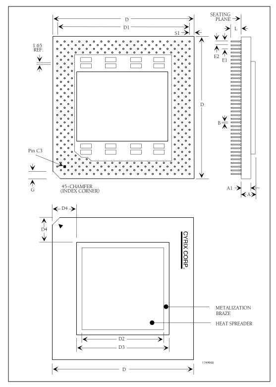
Figure 5-3. 296-Pin SPGA Package
