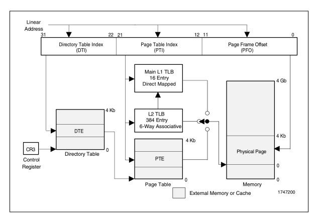
Figure 2-29. Paging Mechanism
