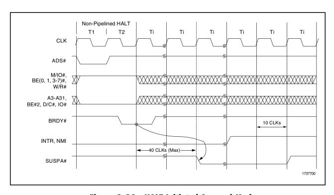
Figure 3-32. HALT Initiated Suspend Mode
