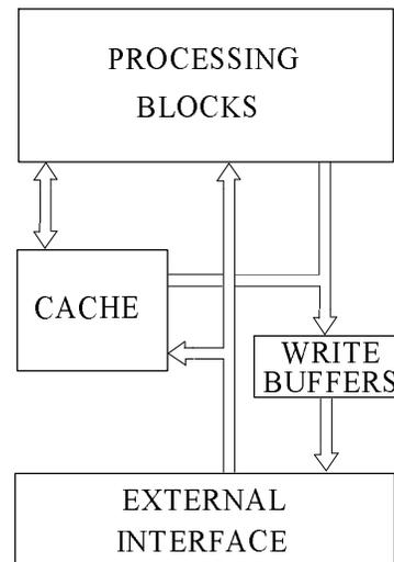
currently stored in the cache. If the data is cacheable and is not currently in the cache, the data is written out to system memory. On the Blue Lightning SX2 and SX3 a line fill request for that physical address is then made. This approach, known as write-allocate, causes
