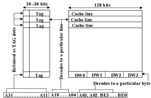
Figure 3: Physical Address Mapping
