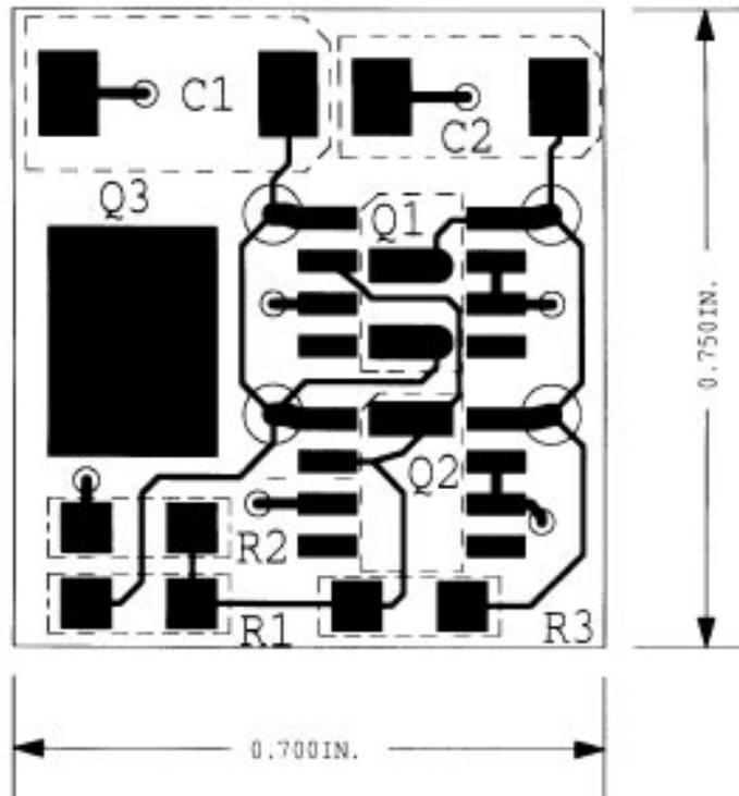
Figure 5: Circuit Layout for 3.3 to 4.2 Volt
