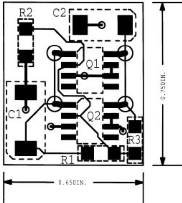
Figure 3: Circuit Layout for 3.6 to 4.2 Volt Regulator
