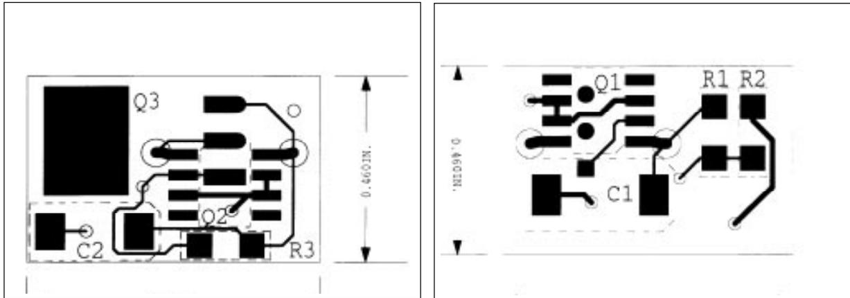
Figures 7A and 7B: Circuit Layout for 3.3 to 4.2 Volt Regulator Using Double Sided Design
